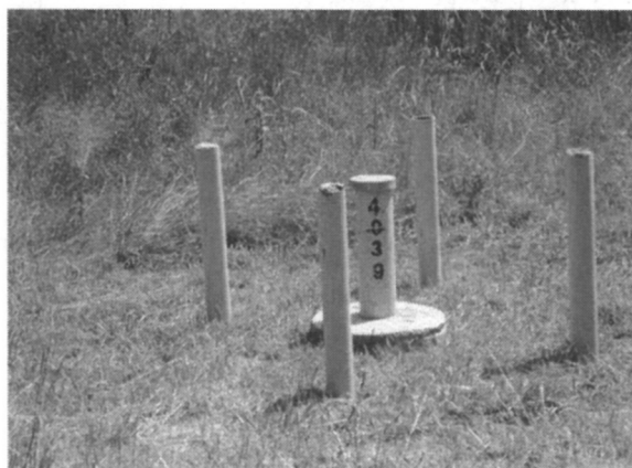
Groundwater monitoring well with protective casings
