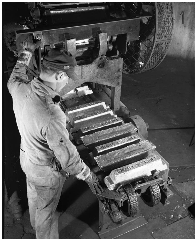
Routine activities at the ASARCO smelter and refinery in 1938. Pouring lead ingots, stamping Omaha & Grant name into cooling ingots, and loading and stacking ingots for shipment. Image from Louis Bostwick and Homer Frohardt, used with permission of The Durham Museum.
