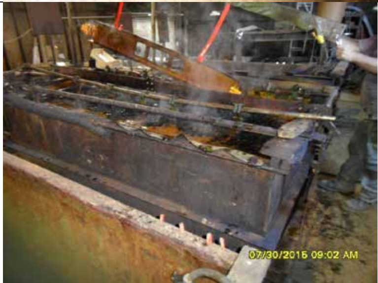
PHOTOGRAPH# 7 DATE TAKEN: 7/30/15 BY: Michael Davis DESCRIPTION: Plating Room- Chrome plating bath.
