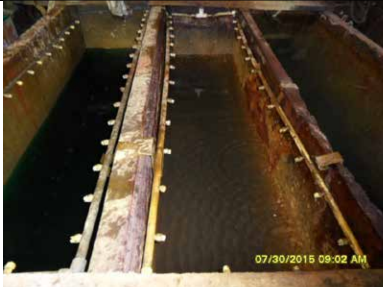
PHOTOGRAPH# 6 DATE TAKEN: 7/30/15 BY: Michael Davis DESCRIPTION: Plating Room- Triple rinse baths following nickel plating
