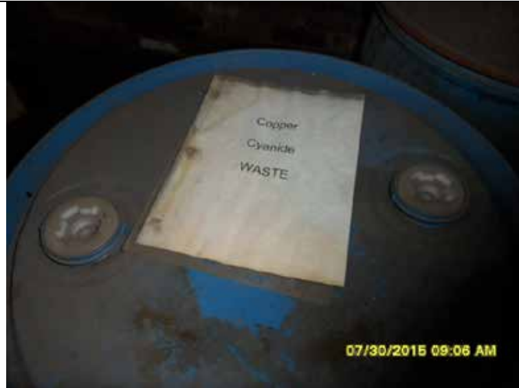
PHOTOGRAPH# 10 DATE TAKEN: 7/30/15 BY: Michael Davis DESCRIPTION: Chemical Storage Area- Label of waste copper cyanide drum. Not labeled "Hazardous waste and no accumulation start date (Violations B9 & B10 in checklist).
