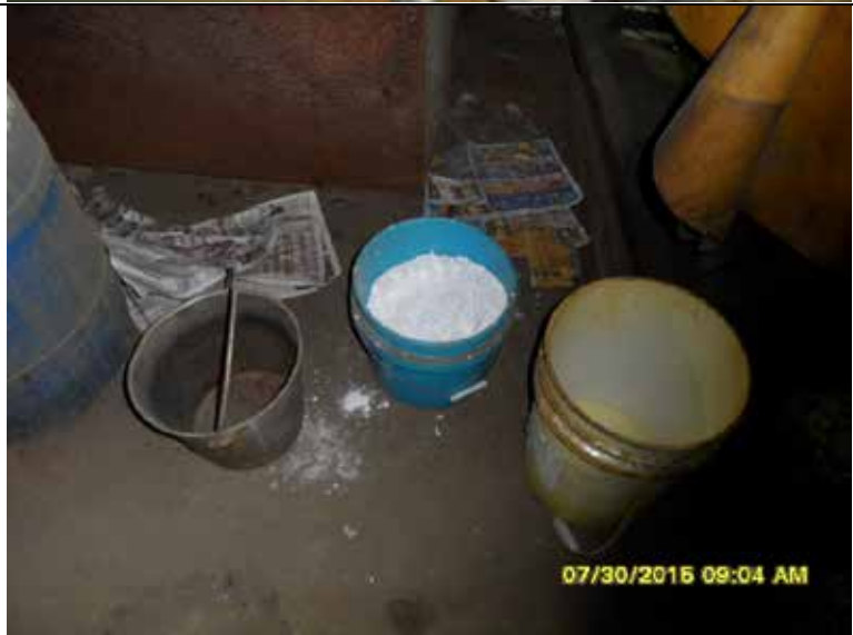
PHOTOGRAPH# 8 DATE TAKEN: 7/30/15 BY: Michael Davis DESCRIPTION: Bucket of absorbent used in case of spills from plating bathes. Several located throughout facility.
