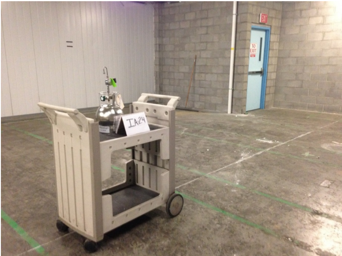
Figure 1: A Typical Indoor Air Sample Setup
