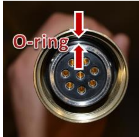
Inside Downhole Cable Logging Head Viton O-ring Size 024 (MINO-8-CCPL) McMaster Carr 9464K78; $9.09/50pcs.
