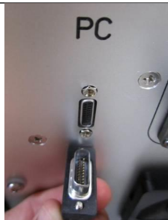
Data Cable Connection on Surface Station
