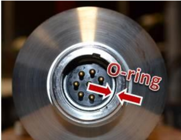
Inside Down Hole Probe Logging Head Viton O-ring Size 023 (MINO-8-BCRL) McMaster Carr 9464K77; $8.06/50pcs.
