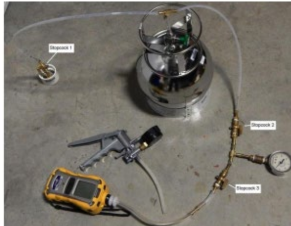
Figure 5: Example 2 Water dam, vacuum leak check and sampling configuration (typ)
