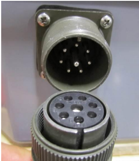
Reference Channel Cable connection to Reference Coil box.
