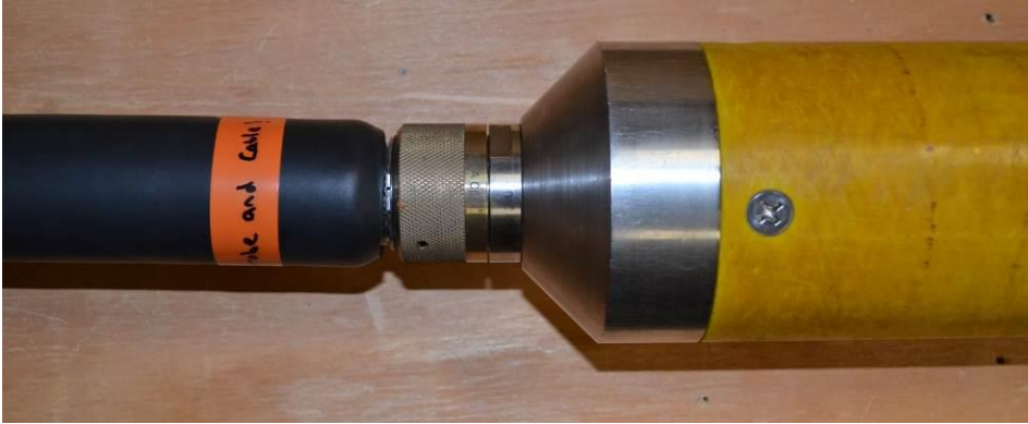
Downhole Probe connected to Logging Cable
