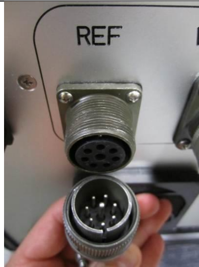
Reference Channel Cable connection to Surface Station.
