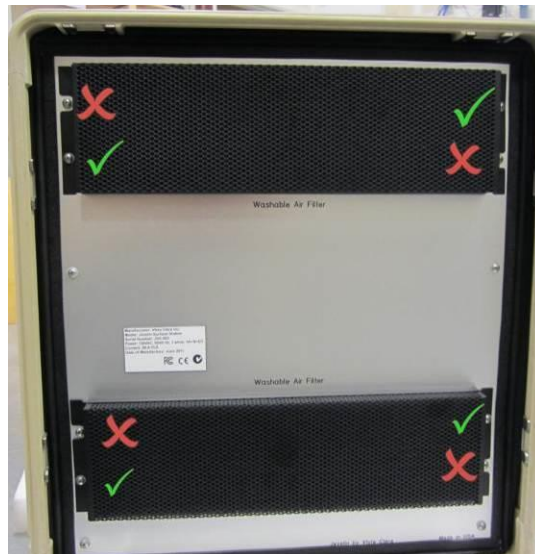
Washable Air Filter Covers on Back Panel of Surface Station. Only remove screws where indicated by green check marks. Do not remove other screws.
