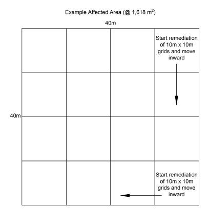
The soil would be excavated from the boundary inward, allowing movement of the hauling equipment closer to the excavator to try to increase efficiency and prevent the spread of contamination.
