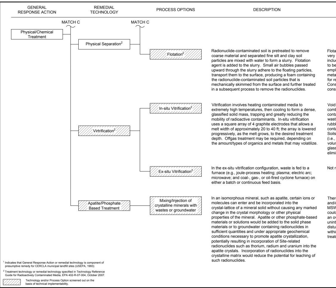
Flotation is most effective at separating soil particles in the very fine 0.0004 to 0.004 inch size range. For soils that include a wider range of particle sizes, flotation would need to be combined with other treatment processes. Has been employed extensively in the mining industry to segregate metal-containing fines, but has not been fully demonstrated for reducing the volume of radionuclide-contaminated soil. Consequently, this option was eliminated from further consideration.
