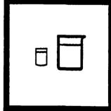
4. Fill a zeroing vial with at least 10 mL of sample (the blank). Collect at least 40 mL of sample in a 50-mL beaker.
