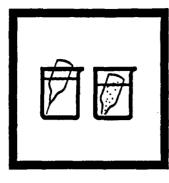
6. Fill a ChromaVer 3 Reagent AccuVac Ampul (the prepared sample) with sample.
