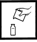
7. Fill another sample cell with 25 mL of sample (the blank).
