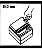
2. Rotate the wavelength dial until the small display shows: 540 nm
