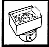
**6.** Place the prepared sample into a boiling water bath.
