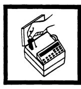
5. Place the AccuVac Vial Adapter into the cell holder.
