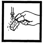
8. When the beeper sounds, remove the prepared sample. Using running tap water, cool the cell to 25°C.
