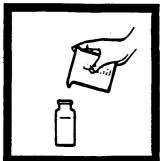
**4.** Fill a clean sample cell with 25 mL of sample.
