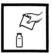
**4.** Fill a sample cell with 25 mL of sample.
