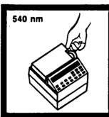
2. Rotate the wavelength dial until the small display shows: 540 nm
