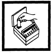
**15.** Place the prepared sample into the cell holder. Close the light shield.
