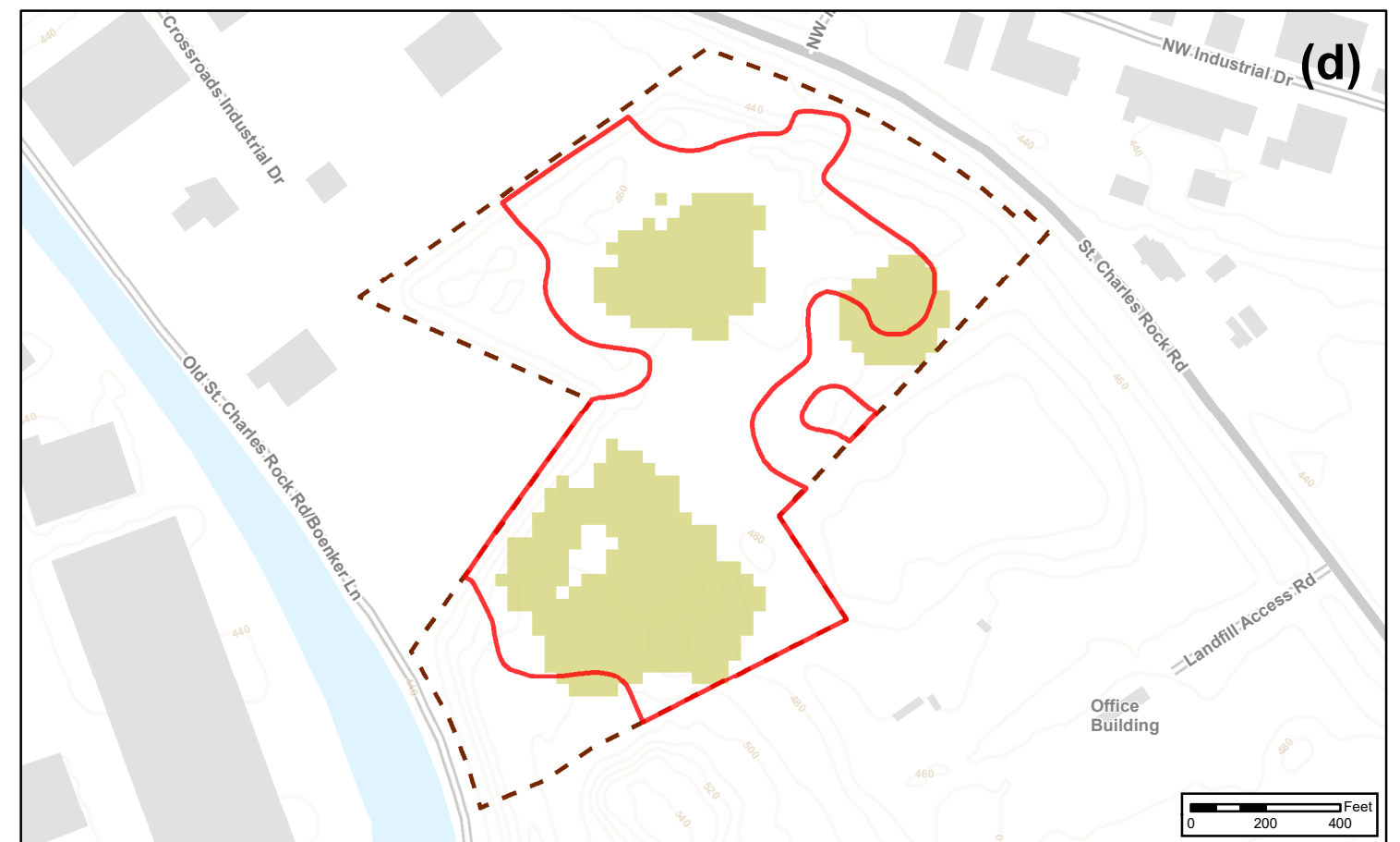
Figure 13 Estimated Lateral Extent of Excavation, Area 2 - Initial Best Estimate: (a) > 7.9 pCi/g, (b) > 52.9 pCi/g within 16 ft of 2005 ground surface, (c) > 500 pCi/g, (d) > 1000 pCi/g
