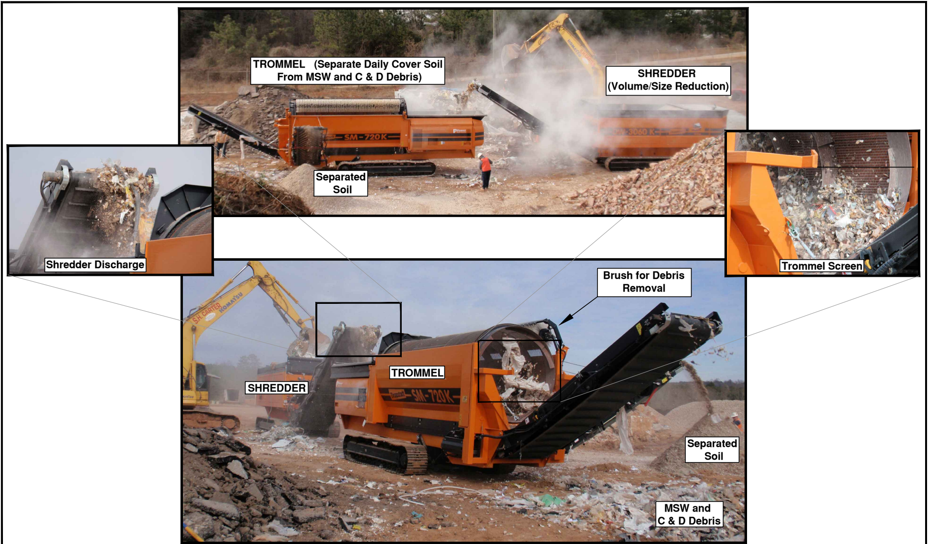
Figure 4-2 Waste Volume/Size Reduction and Separation Equipment West Lake Landfill OU-1 Final Feasibility Study EMSI Engineering Management Support, Inc.
