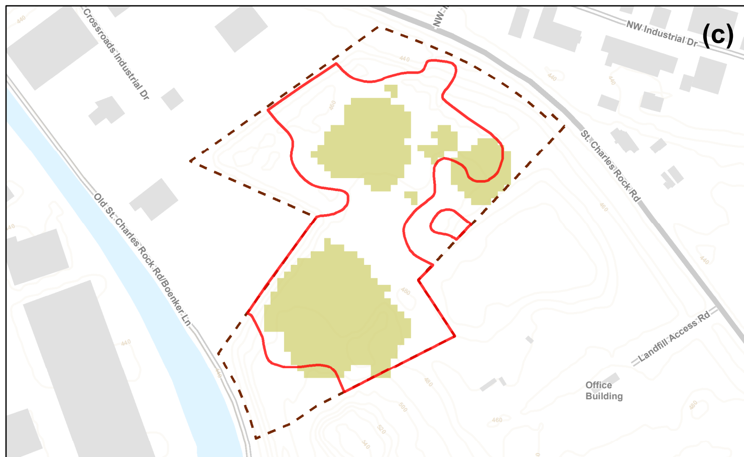
Figure 13 Estimated Lateral Extent of Excavation, Area 2 - Initial Best Estimate: (a) > 7.9 pCi/g, (b) > 52.9 pCi/g within 16 ft of 2005 ground surface, (c) > 500 pCi/g, (d) > 1000 pCi/g
