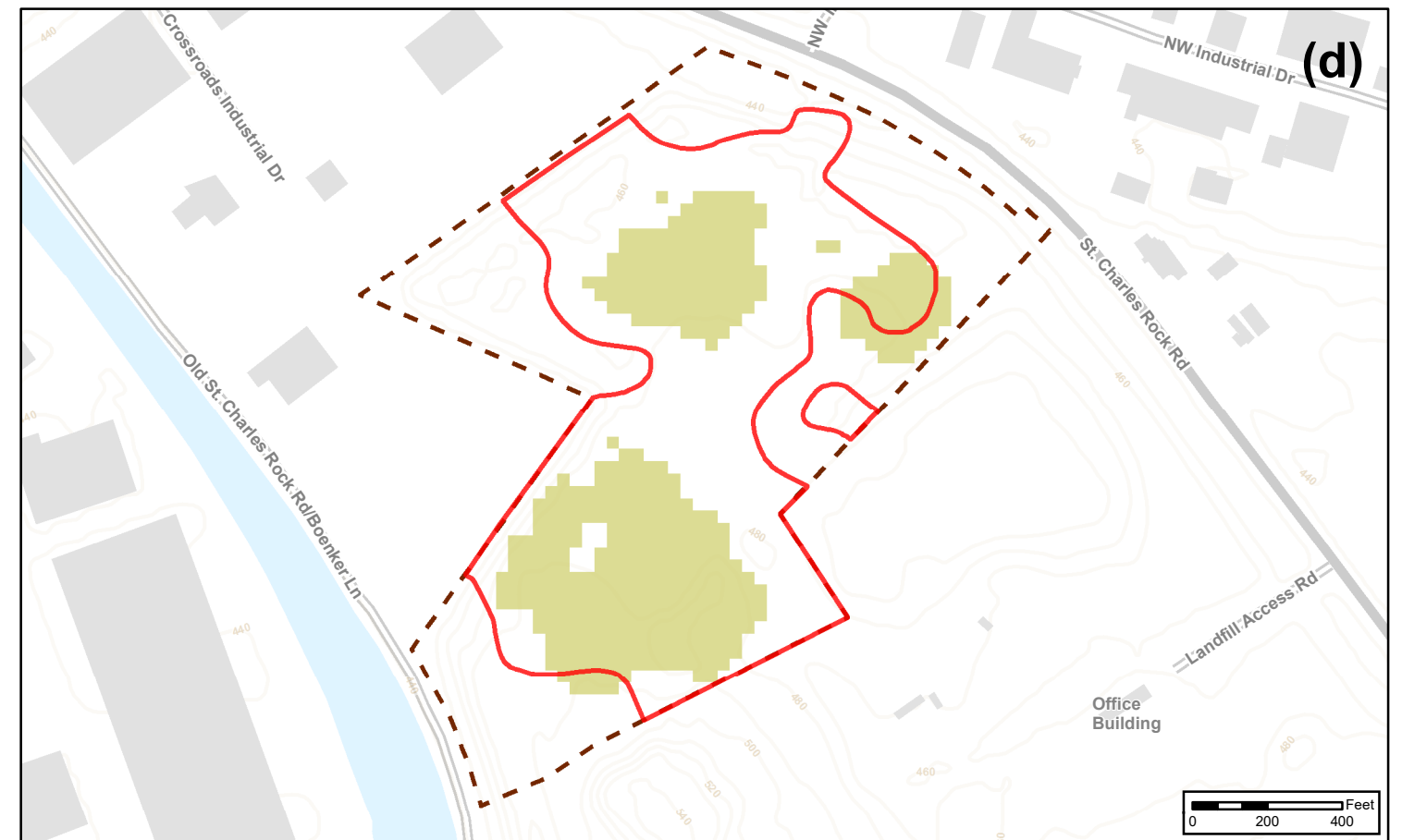
Figure 17 Estimated Lateral Extent of Excavation, Area 2 - Updated Best Estimate: (a) > 7.9 pCi/g, (b) > 52.9 pCi/g within 16 ft of 2005 ground surface, (c) > 500 pCi/g, (d) > 1000 pCi/g
