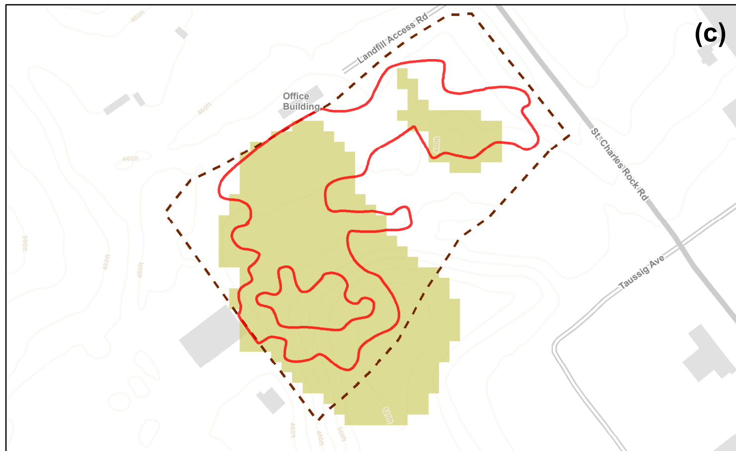
Figure 16 Estimated Lateral Extent of Excavation, Area 1 - Updated Best Estimate: (a) > 7.9 pCi/g, (b) > 52.9 pCi/g within 16 ft of 2005 ground surface, (c) > 500 pCi/g, (d) > 1000 pCi/g
