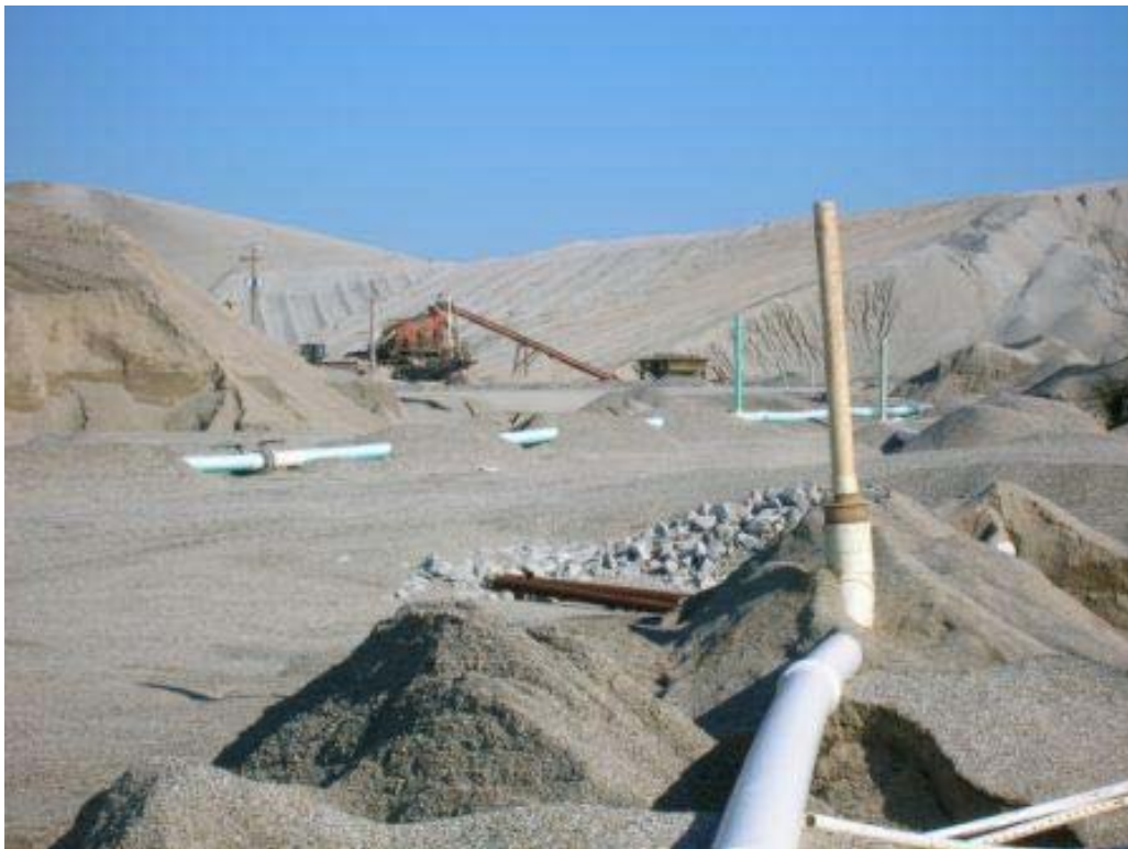
Photo 66: Chat washing unit at the Sooner Chat Pile.
