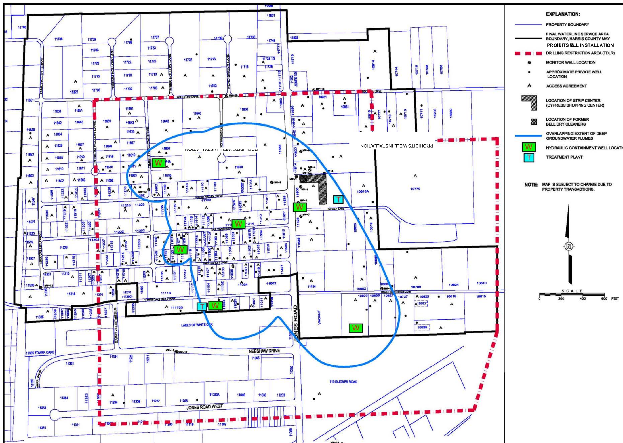
Figure 10 – Hydraulic Containment / Pump and Treat
