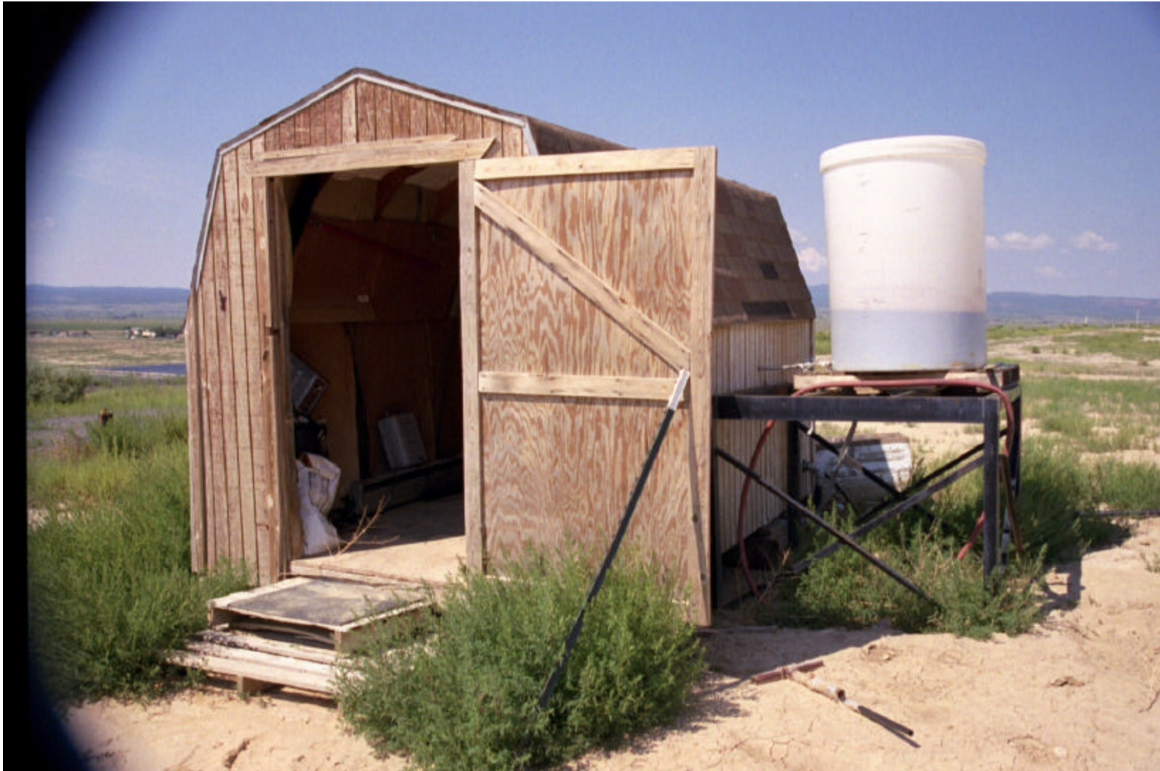
Bioremediation experiment station on top of large tailings pile (location visible in previous photograph). Injection well is located inside structure; molasses additive is in white tank. Associated monitoring wells are left of the structure.
