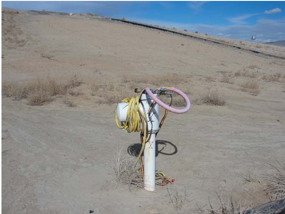
Photo 13: Point-of-Compliance (POC) Well X at the toe of the small tailings pile. The well was installed in 1975 and monitors the base of the alluvium at approximately 51 feet below ground surface. View looking northeast.
