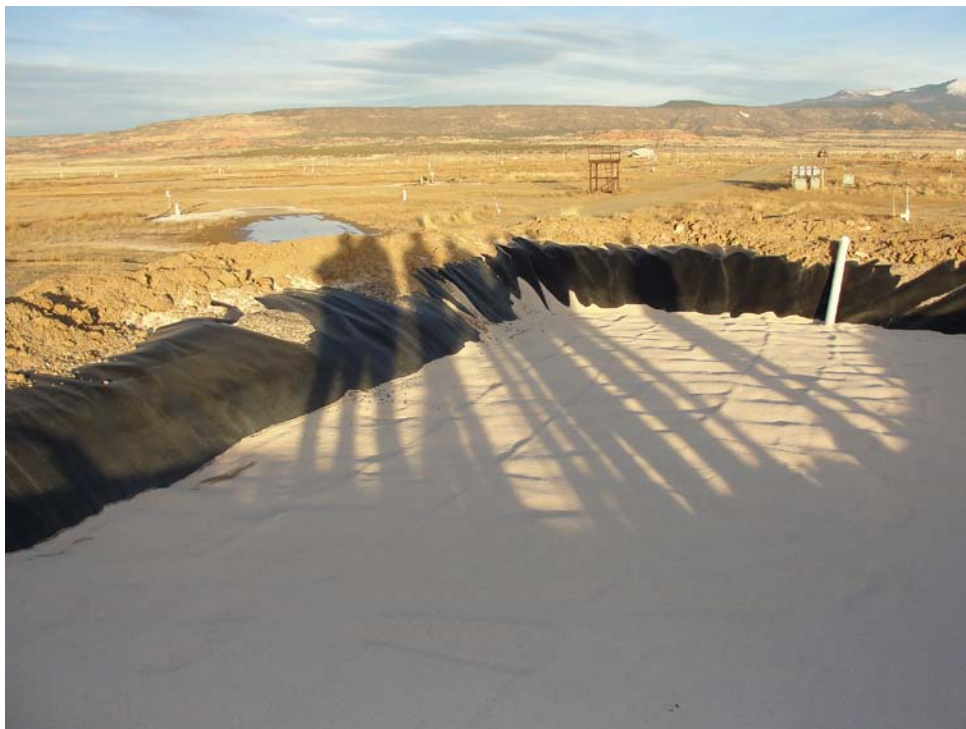
Photo 8: Zeolite pilot-test pit on the top of the large tailing pile. The zeolite is used to extract low-concentration uranium before being re-injected at 50 gallons per minute. Pit is lined with a 60 millimeter thick high density polyethylene (HDPE) liner. View looking northeast.
