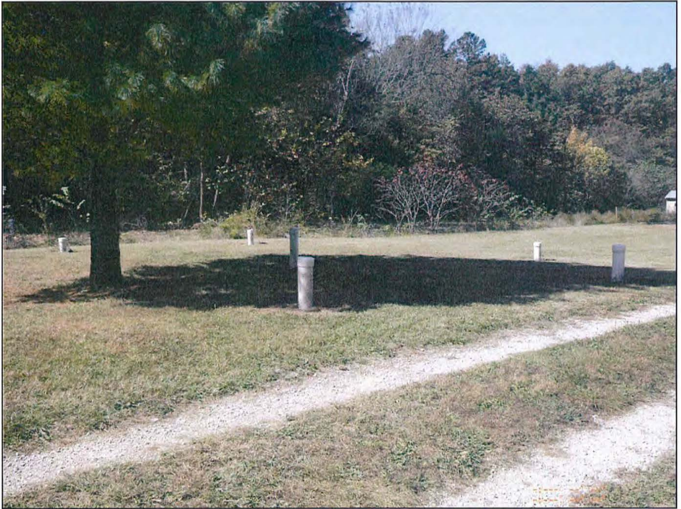
Photo 5: Site Former Sinkhole Area With Injection Wells
