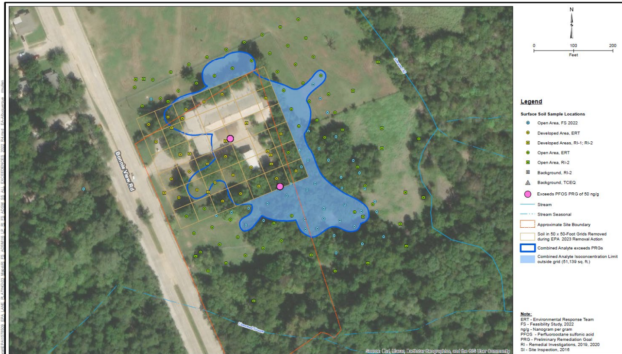
Figure 3 Map of the Area with Lead, Mercury, Arsenic, and Hexavalent Chromium Levels Above PRGs in Soil
