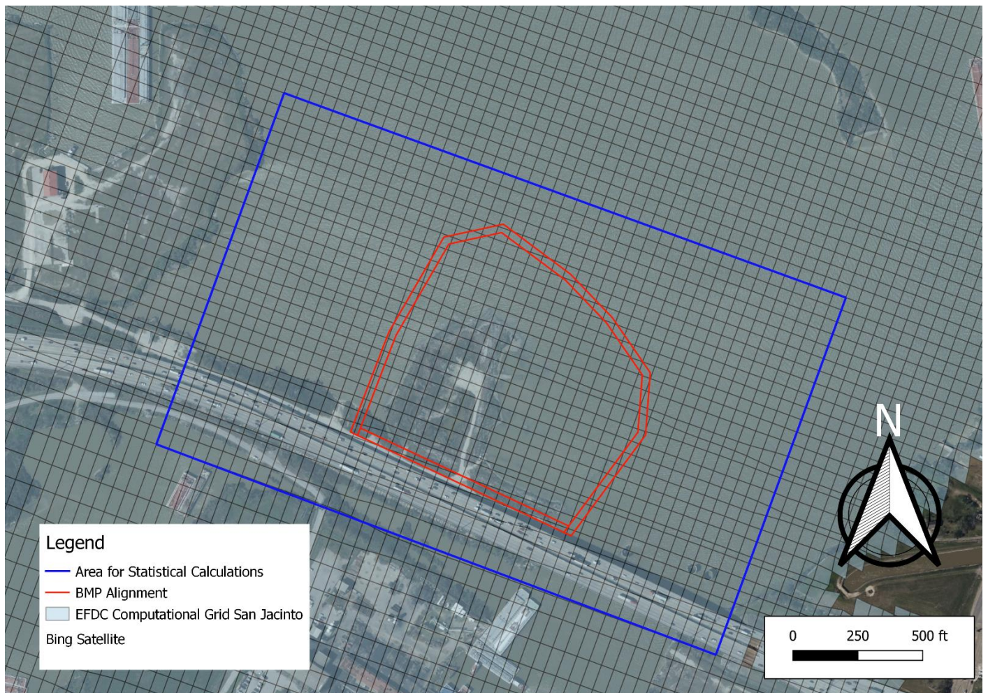
Figure 23 Area Used for the Computation of Statistics for the Conditions Around the Cofferdam
