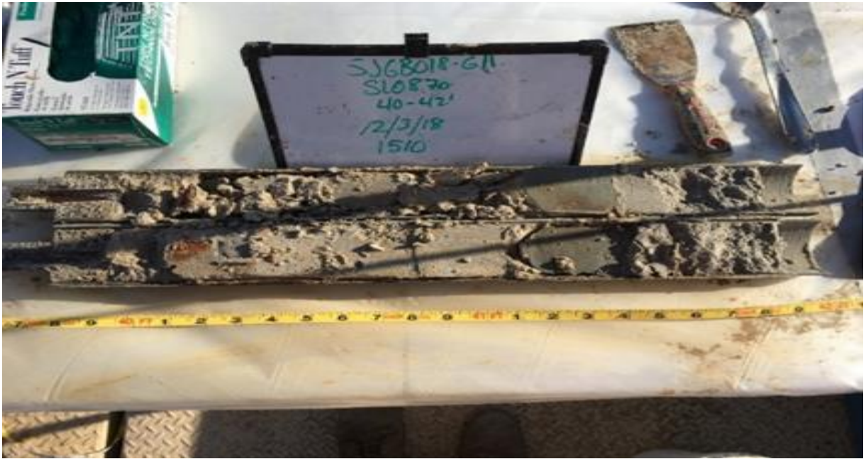
Photo 1 Figure D.1: Sample G11 (40 to 42 feet (ft) deep in borehole SJGB-018).
