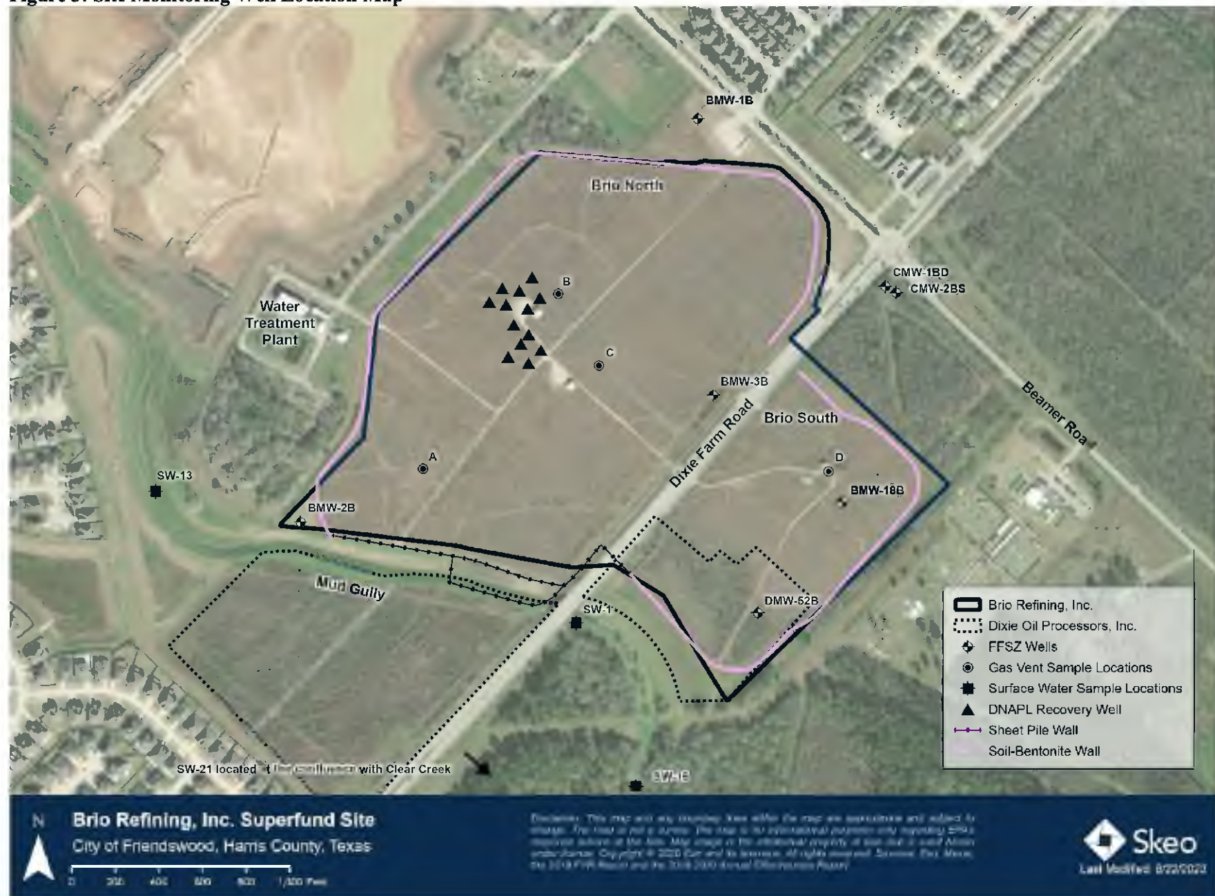
Figure 3: Site Monitoring Well Location Map
