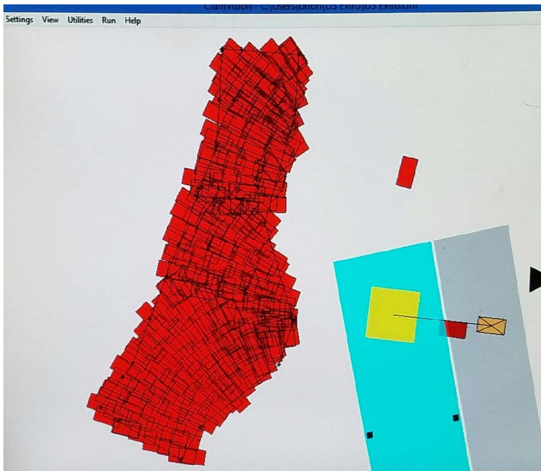
Photograph 4: Crane Tip GPS system. Shows total bucket coverage with first rock pass
