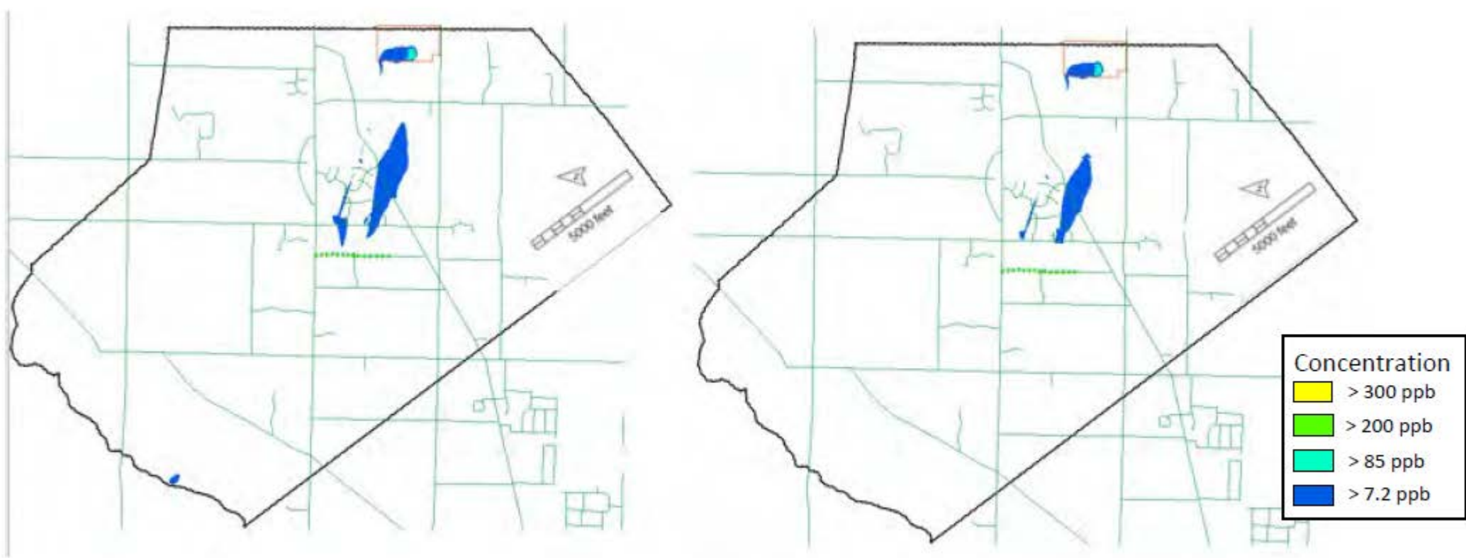
Figure 17c, d – Model Simulated 1,4-DD Results: P&T at Skyview Drive at 40 (2062) and 50 (2072) years.
