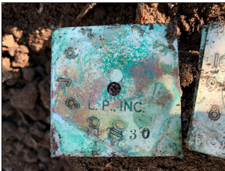
A radioactive backing of a clock produced by Luminous Processing, Inc. for Westclox excavated by the Illinois Emergency Management Agency during the previous remediation.
