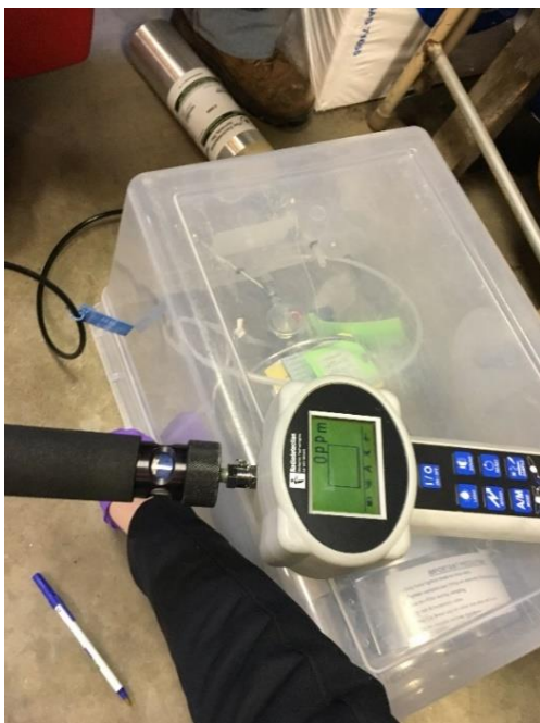
Figure 6-6. Helium Leak Test Using Shroud
