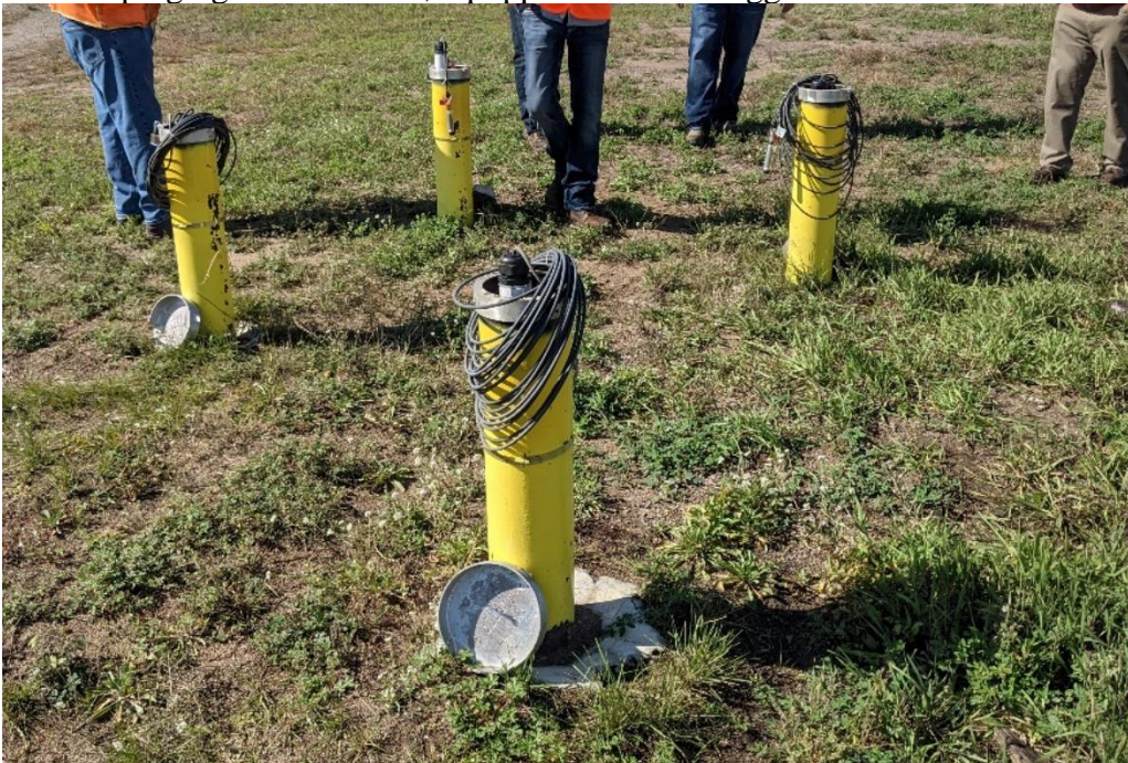
Figure D-14: Monitoring well nest MW-41 (MW-41AA/A/B/C), constructed to evaluate in-situ biosparging effectiveness; equipped with data loggers.
