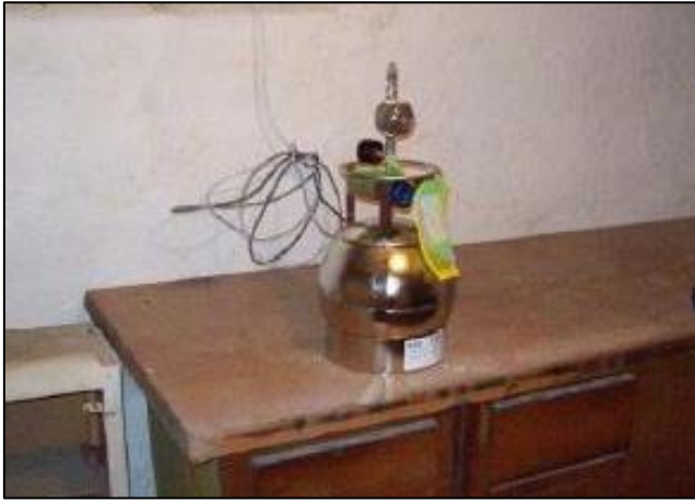
This photo shows a Summa canister, which is left in place for 24 hours to collect samples of indoor air. The silent device is about the size of a basketball.
