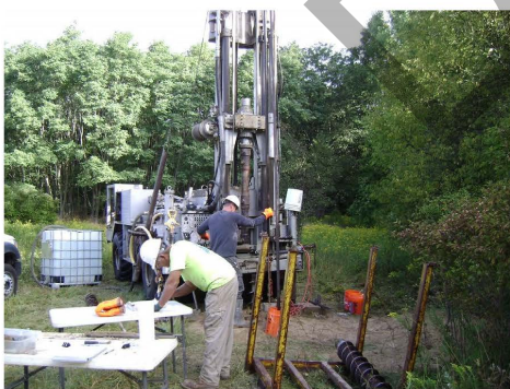
Contractors use a Geoprobe to collect soil samples on the Wolverine site.
