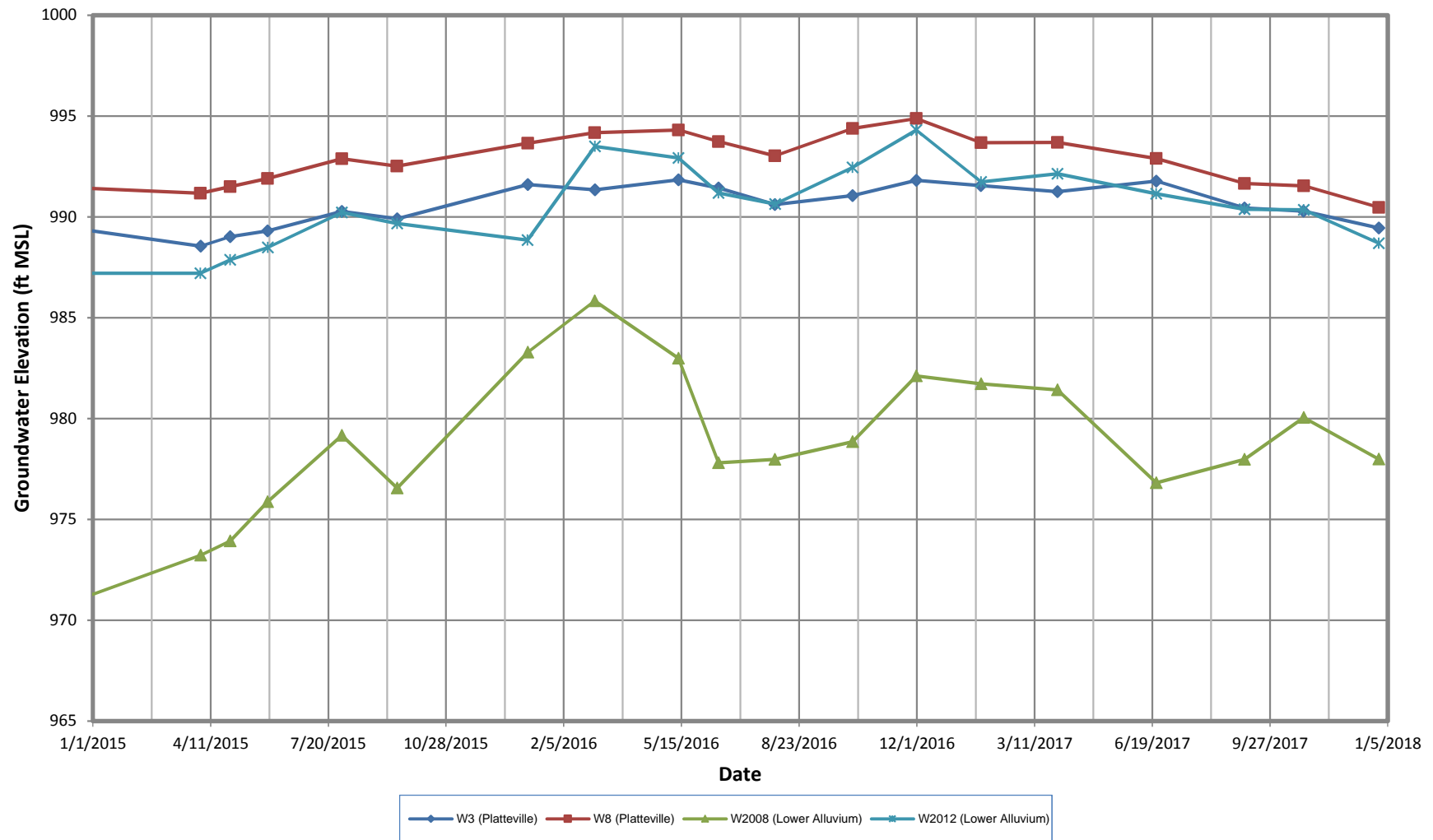
Figure 3-4 Hydrograph of Platteville (W3 and W8) and Lower Alluvium Wells (W2008 and W2012) January 2015 - December 2017 Oakdale Site, Oakdale, MN
