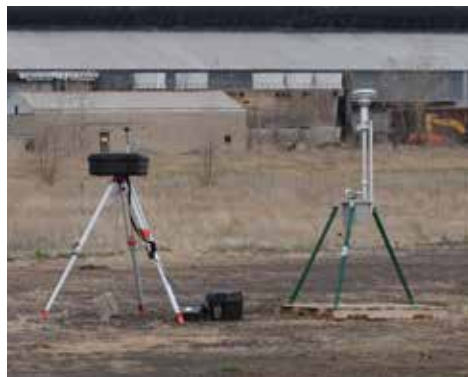
Perimeter air monitors.
