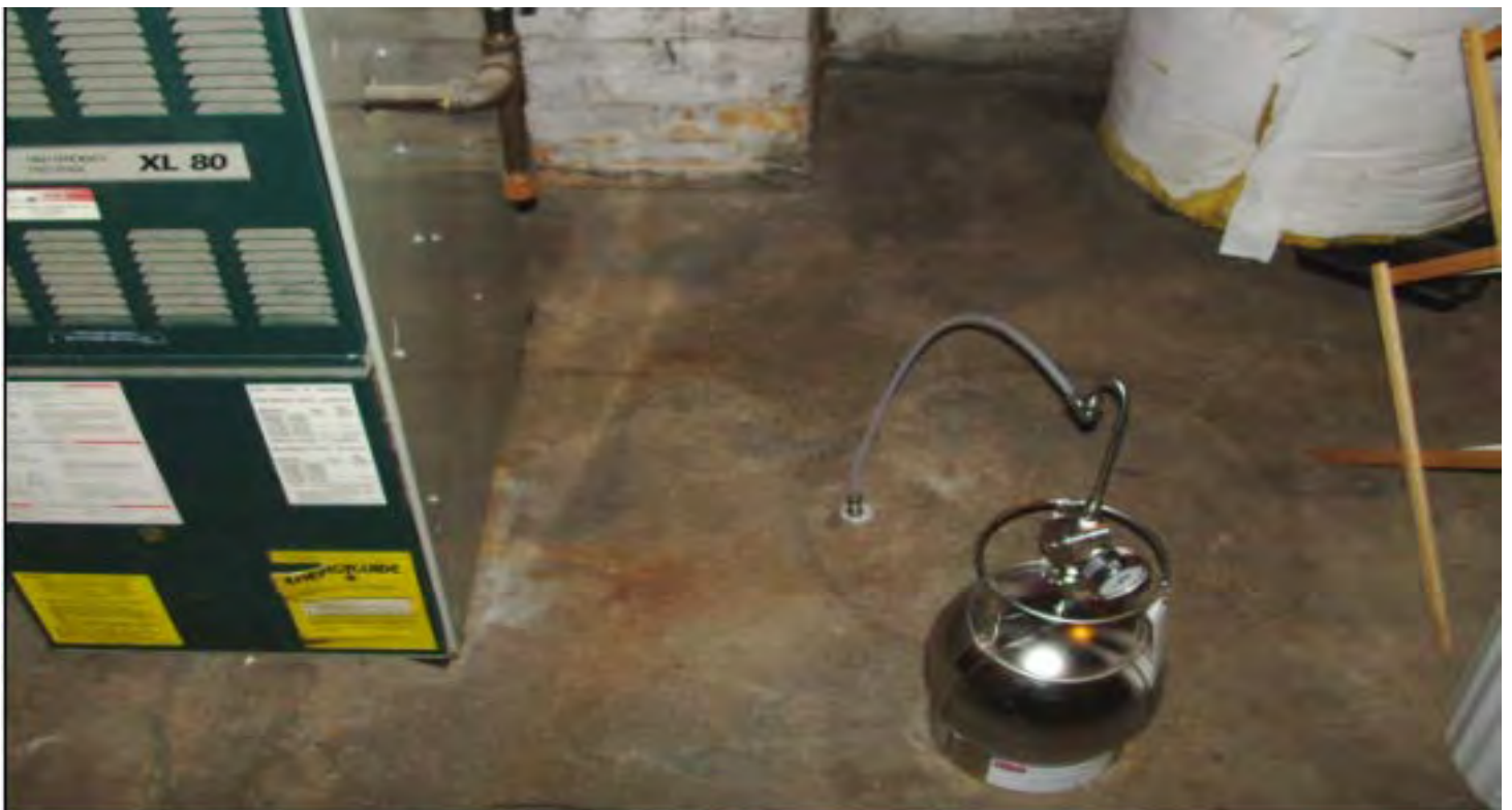
Canisters like this will be placed in basements to collect sub-slab air samples.
