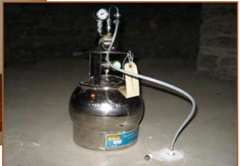
Canisters like this were placed in basements to collect sub-slab air samples.
