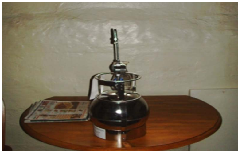
Canister used to collect indoor air samples inside a house.
