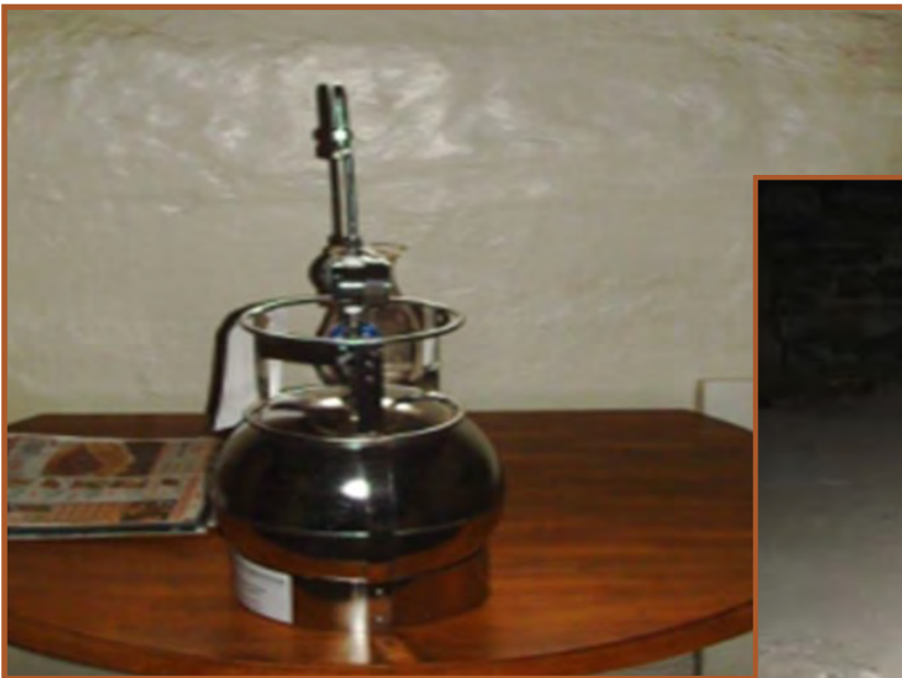
Canister used to collect indoor air samples inside a house.
