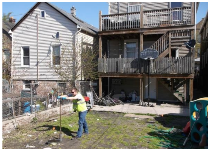
Taking a soil sample is a simple and routine process. This investigator is seen using a hand auger to dig a small hole in the soil that can be collected for laboratory analysis.
