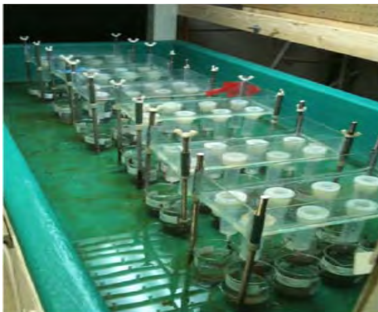
Figure 2-1 Sediment Toxicity Test Exposure System at ERDC Laboratory.
