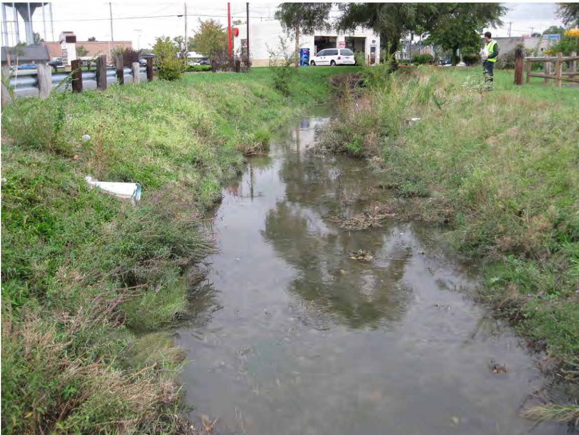
Amlosch Ditch Photo 5: Sample station in Amlosch Ditch, depicting little to no bank erosion, high channel stability and little to no instream cover.
