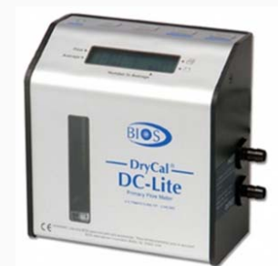
Flow rate calibration unit
