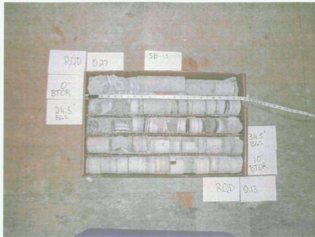
1. PHOTOGRAPH OF BEDROCK CORES COLLECTED FROM THE KOKOMO LIMESTONE 24.5 TO 34.5 FEET BELOW GRADE AT BORING SB-13/MW-13 THAT SHOW VERY POOR ROCK QUALITY WITH RQDs OF 13% TO 27%.
