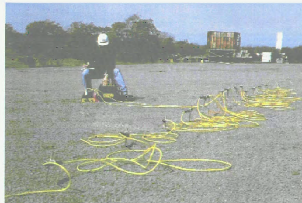
PHOTO 2. TYPICAL ERT ARRAY SETUP
