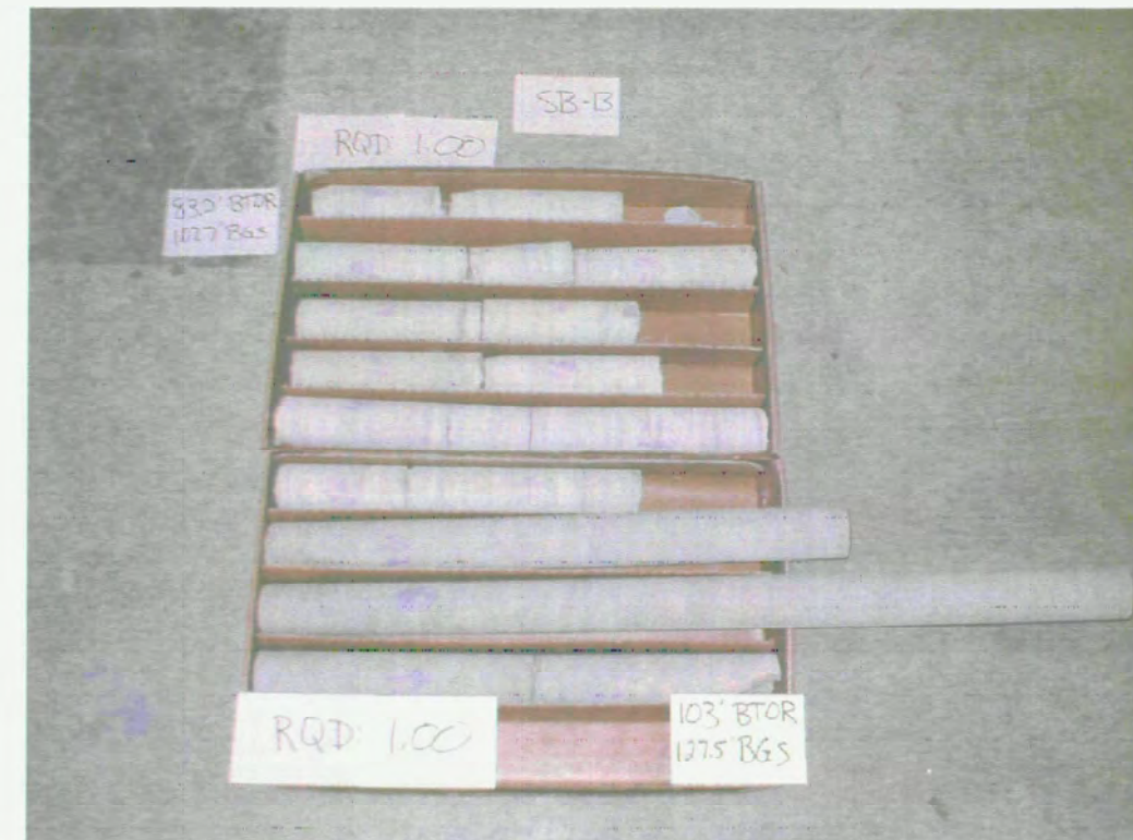
2. PHOTOGRAPH OF BEDROCK CORES COLLECTED FROM THE MISSISSINEWA SHALE 107.5 TO 127.5 FEET BELOW GRADE AT BORING SB-13/MW-13 THAT SHOW EXCELLENT ROCK QUALITY WITH RQDs OF 100%.
