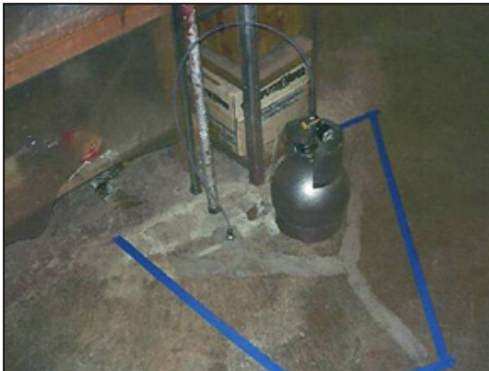
Sub-slab sampling canister and probe.
