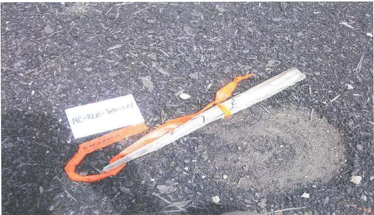
Charred debris that tested positive for asbestos
