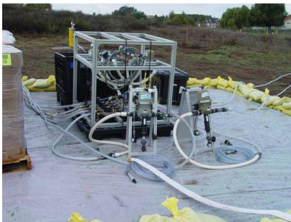
Figure 5.11 Proportional Feed System for a 10-Line Injection System (Photo courtesy of Remediation and Natural Attenuation Services, Inc.)
