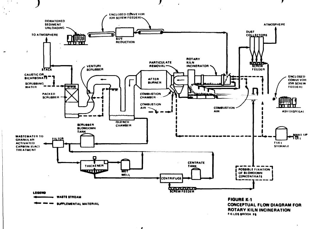
the solids retention time, which can be as long as 60 minutes.
