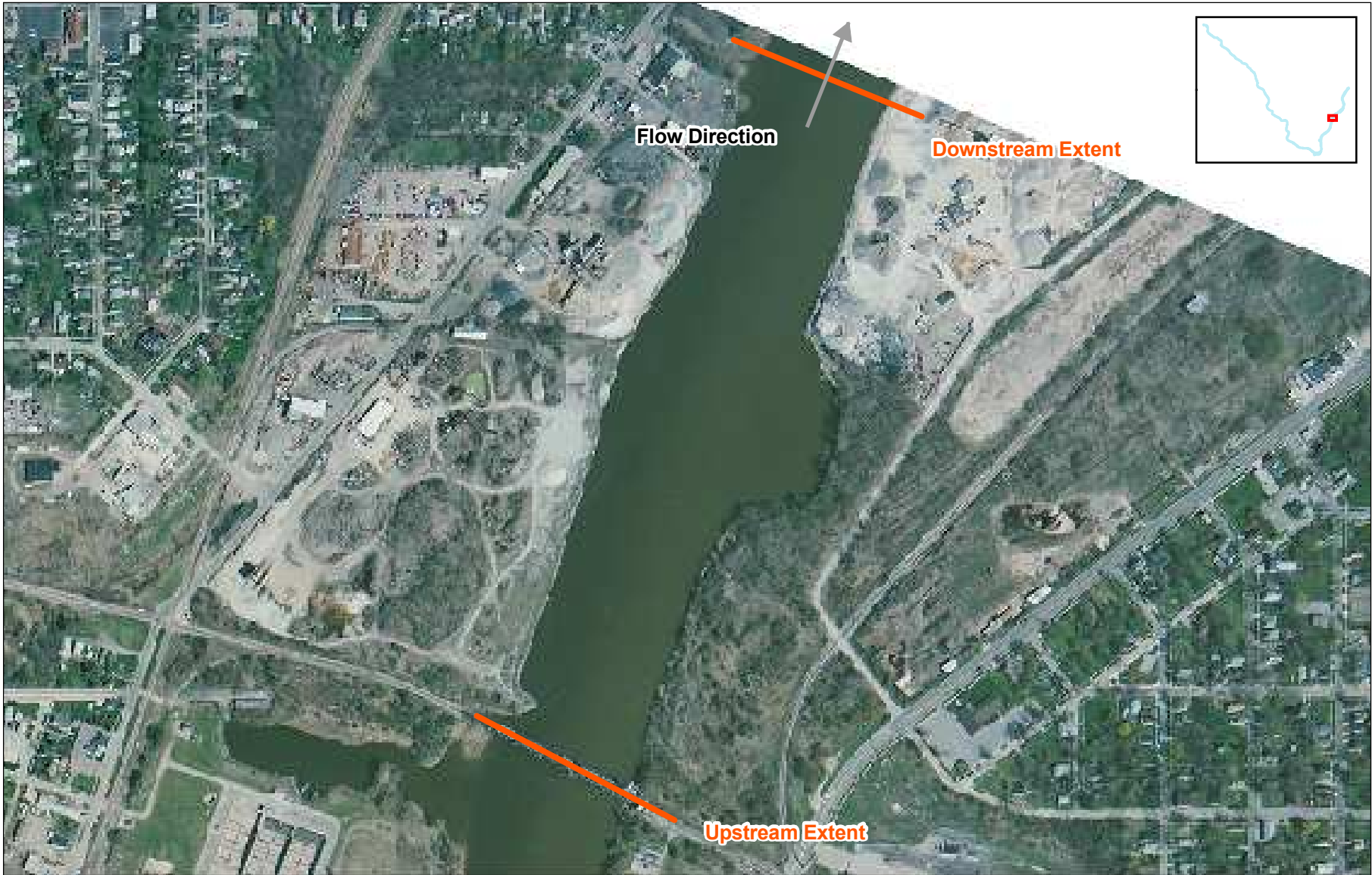
Approximate Bathymetric Surveying Locations for Sixth Street Turning Basin
