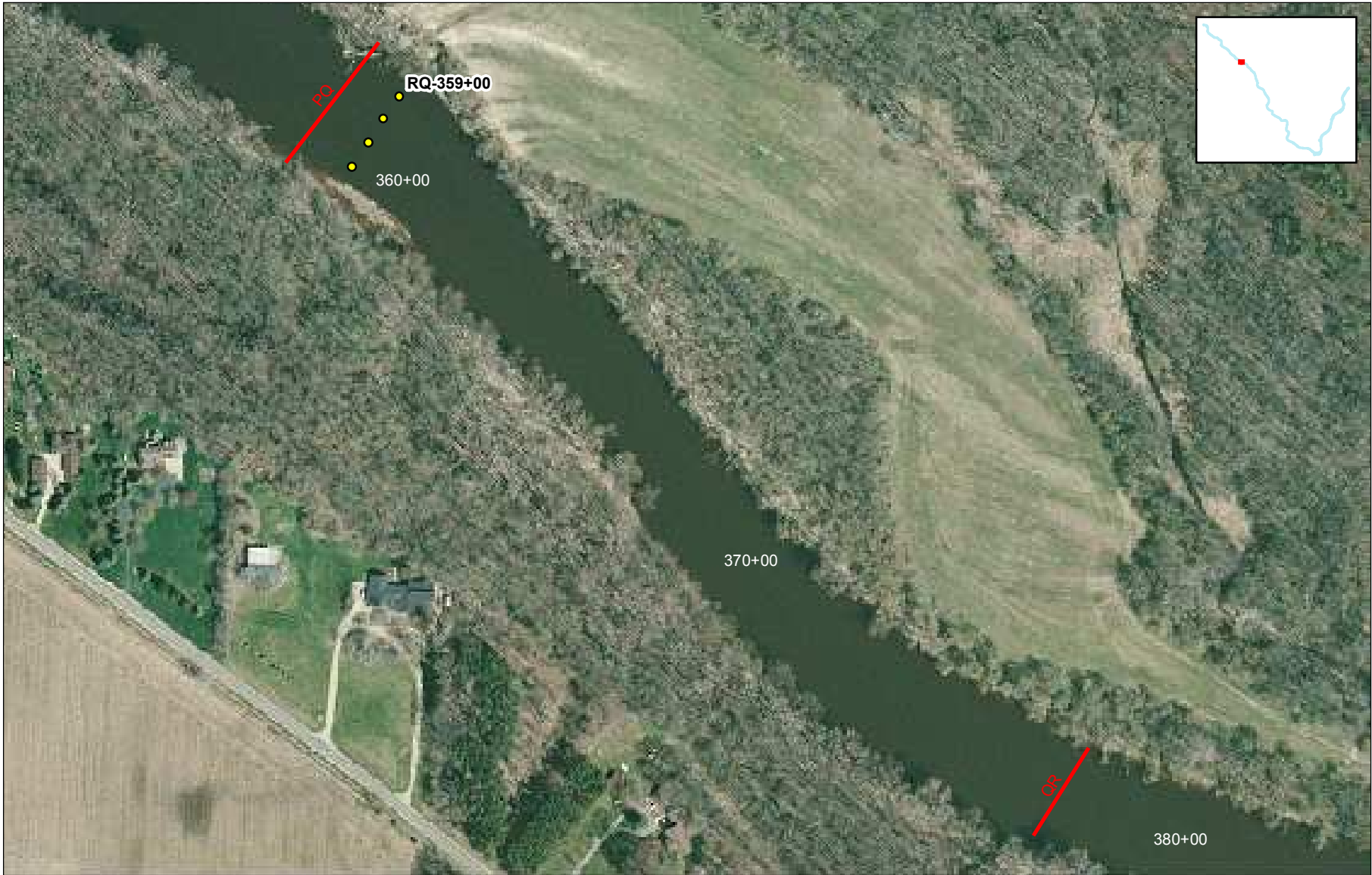
Approximate In-Channel Bed Pin Monitoring Locations Reach Q
