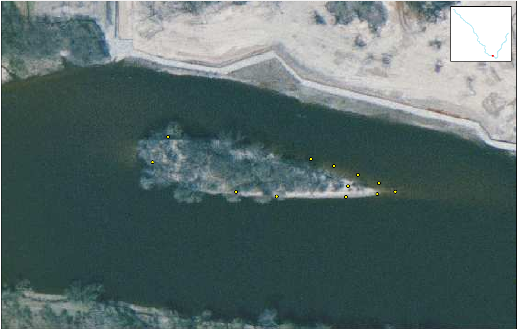
Approximate Topographic Surveying Locations for Reach WW In-Channel Center Island
