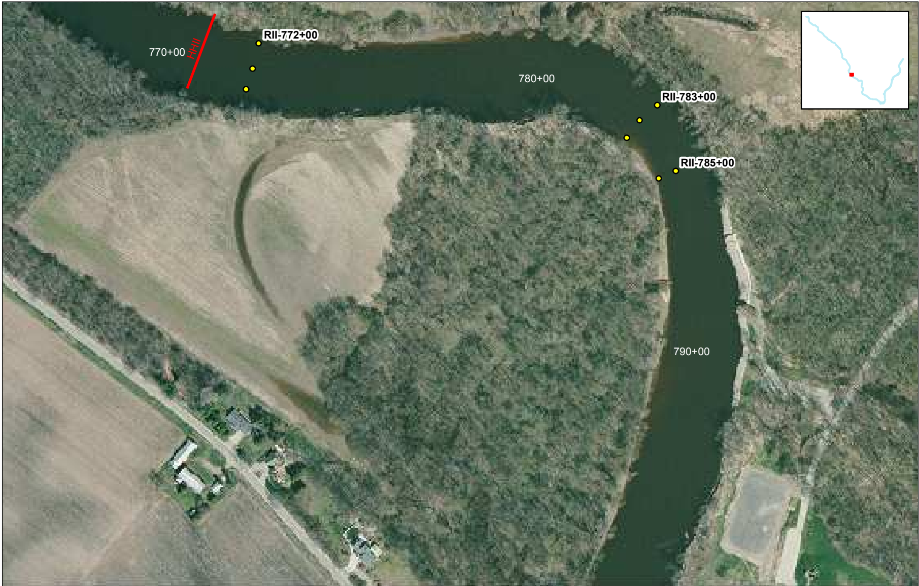
Approximate In-Channel Bed Pin Monitoring Locations Reach II (Upper)
