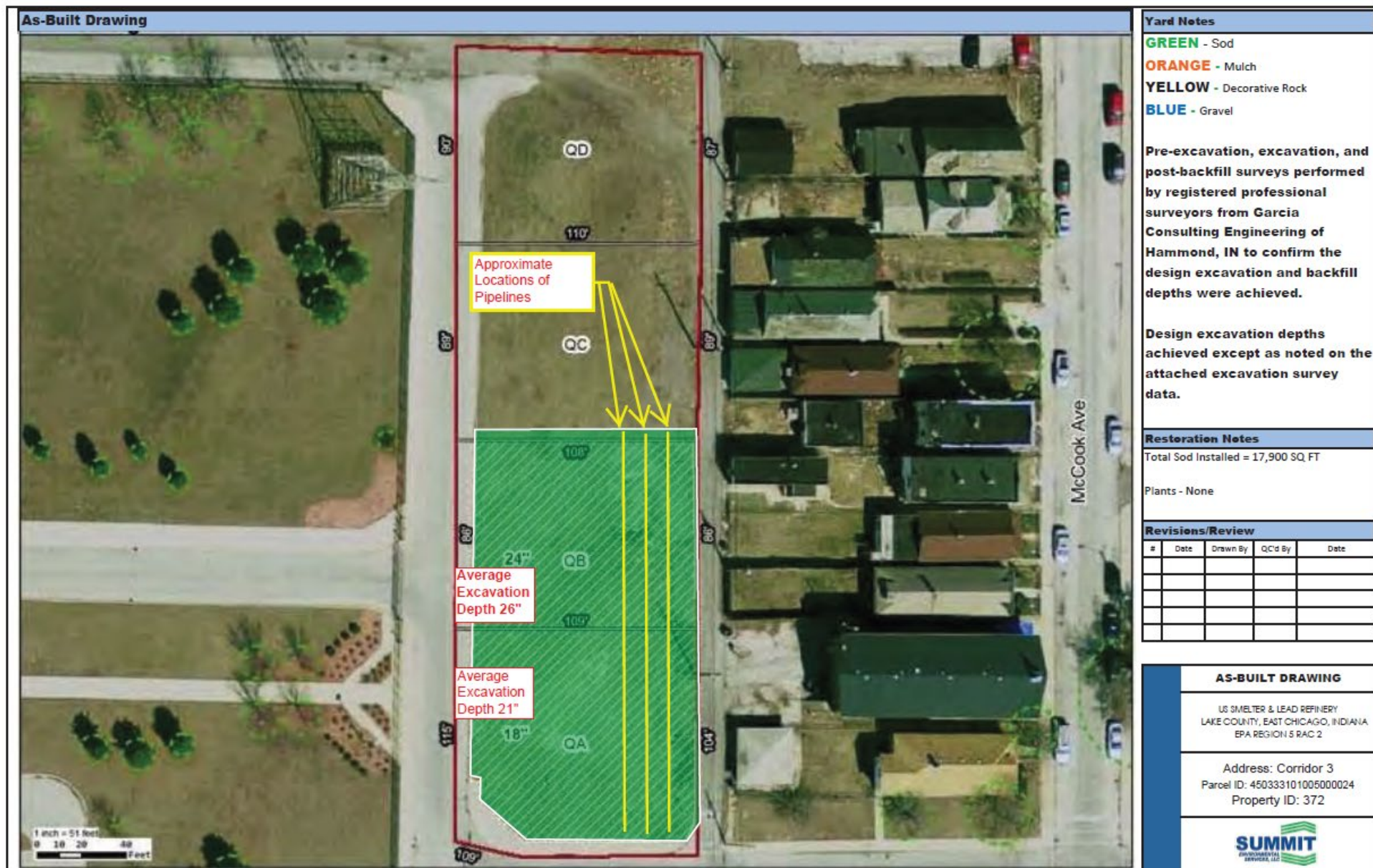
FIGURE 12: Zone 1 Corridor 3 Property Remedial Action As-Built Drawing
