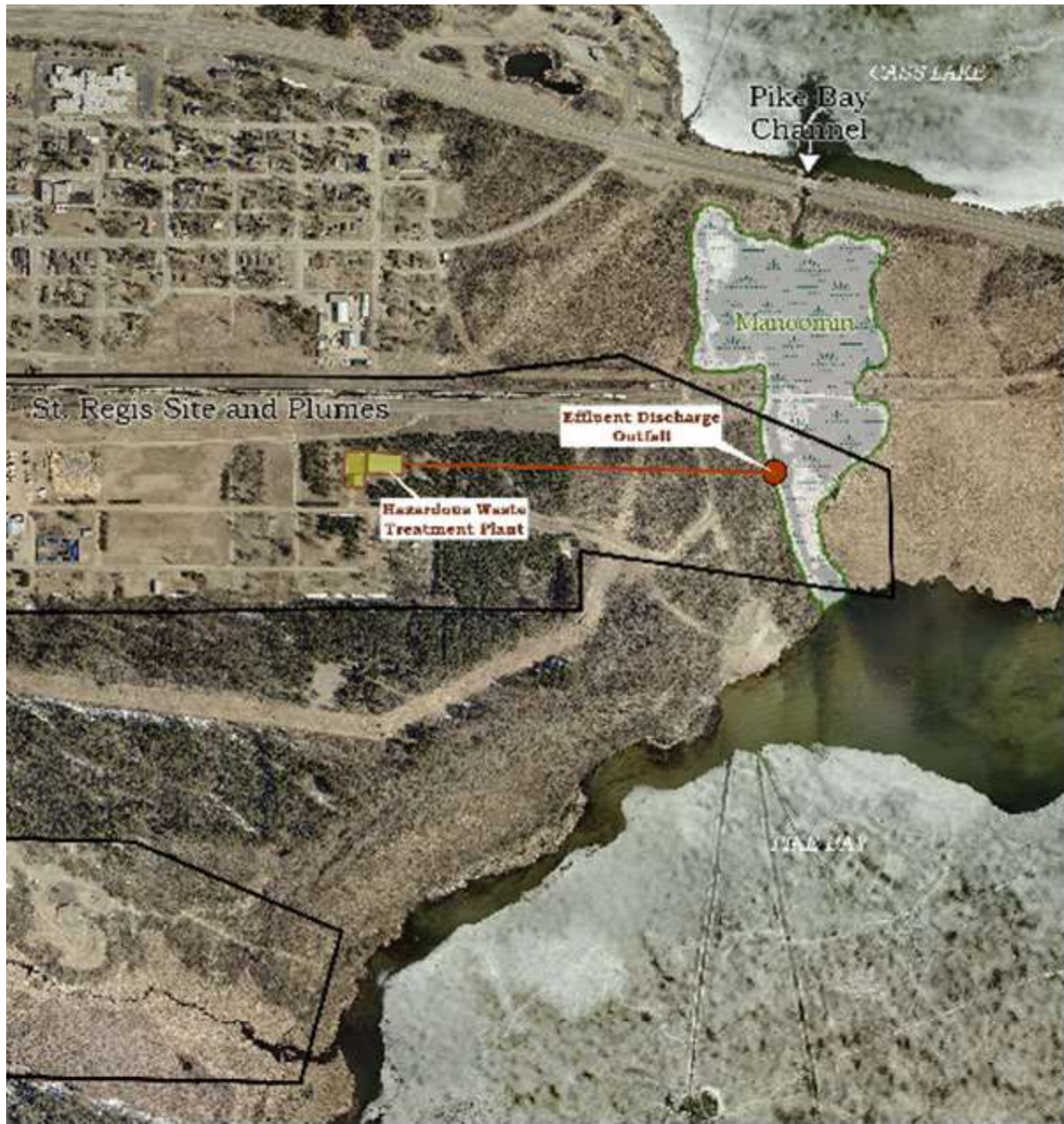
Map showing St. Regis contaminant plumes, treatment plant, effluent discharge outfall, and Pike Bay Channel wild rice bed, marked as “manoomin.”
