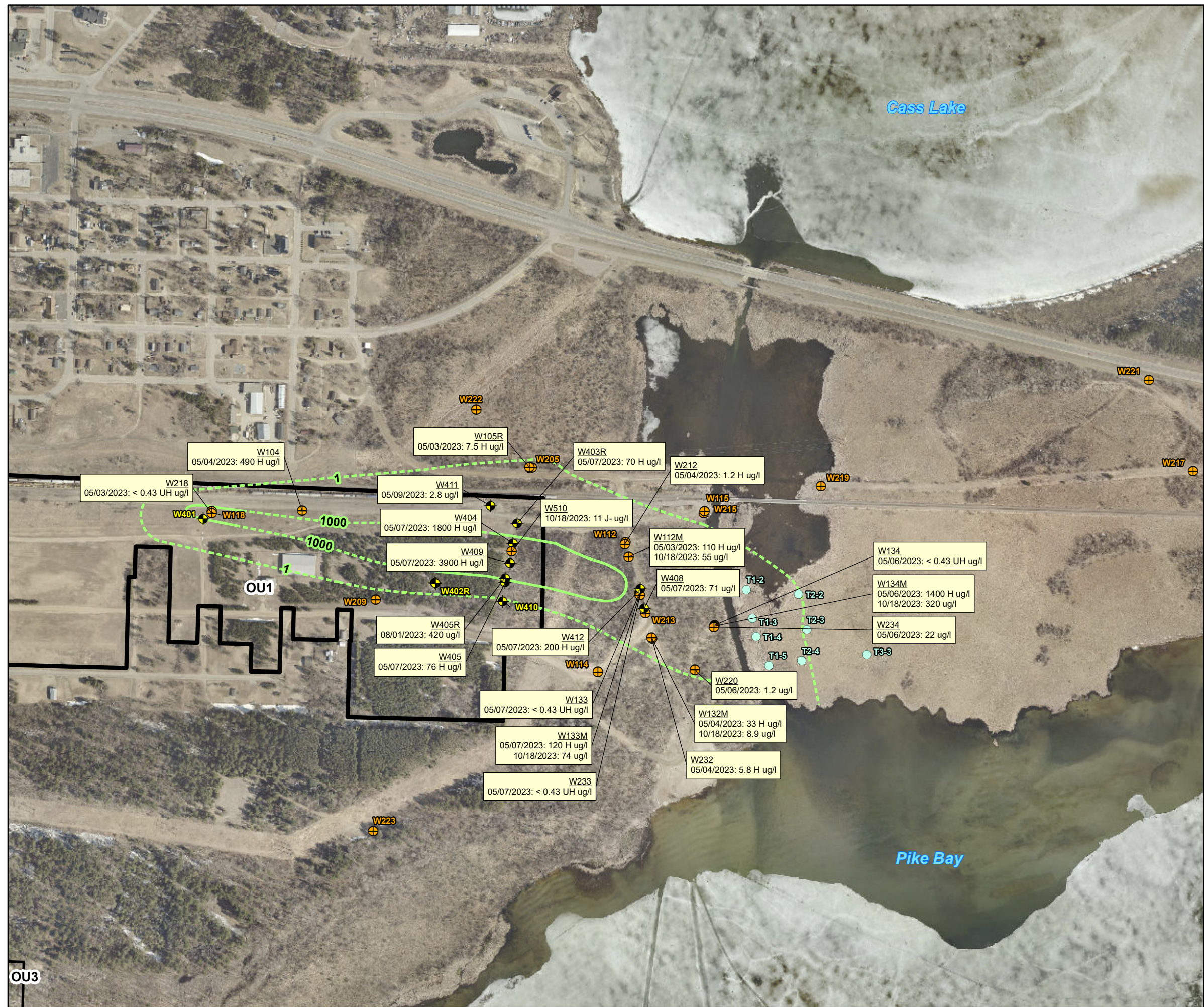
Figure B-6 Current Extents - OU1 PCP Plume Upper Outwash Aquifer Adapted from Figure 3 of the 2024 Annual Report
