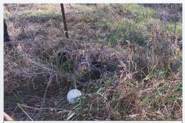
Photograph 10: Unlabeled pipes of unknown construction venting gas at the ground surface near the west fence.
