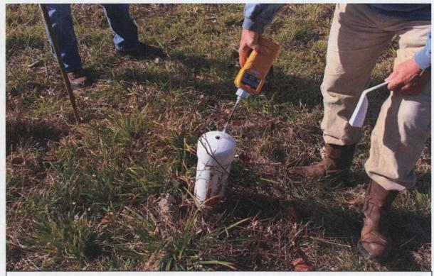
Photograph 11: Unlabeled gas vent of unknown construction with gas above potentially explosive levels near the ground surface (note red light on meter).
