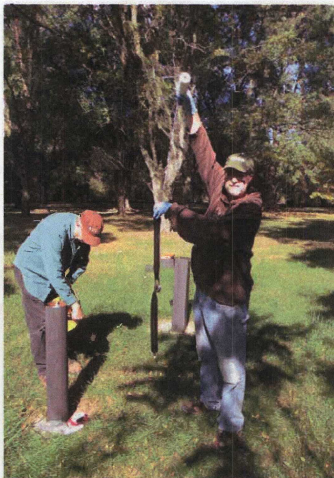
10/14/2013: Deploying passive diffusion samplers in MW-01.
