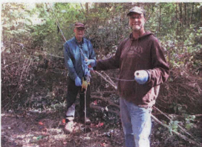
10/14/2013: Deploying passive diffusion sampler in MW-17.
