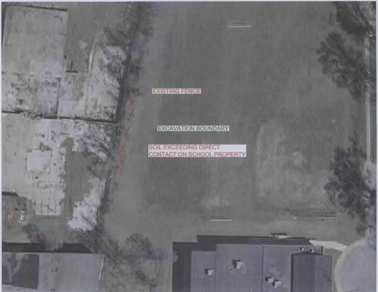
Figure 3. Southeastern portion of the Spartan Chemical Company Site, adjacent school property to the east, site fence, and excavation plans
