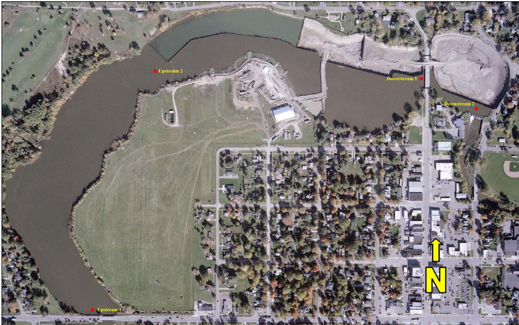
Figure 6. Turbidity Monitoring Locations Velsicol Chemical/Pine River Site in St. Louis, Michigan OU2 Remedial Action - 2006 Cleanup Status Report
