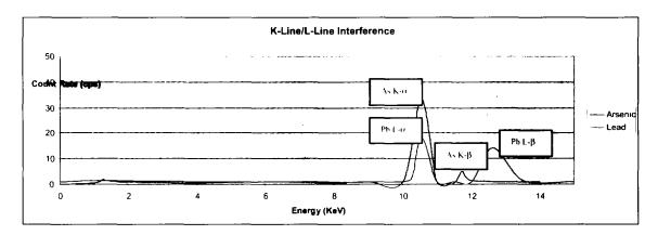
You can see that the K- $\alpha$  peak for arsenic overlaps the L- $\alpha$  peak for lead. This leads to error in elemental analysis. While there will be a degree of uncertainty in the measurements, the XRF is capable of identifying whether the element represented by the peak at 10.5 KeV is lead or arsenic as well as reducing the amount of error in the reported concentrations. There are three techniques that allow the XRF to reduce the error in measurements.
