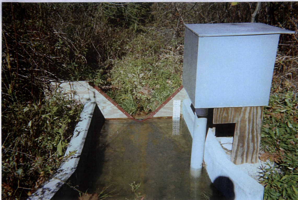
Photograph No. 15 Orientation: North Description: V-notch weir and USGS gage at North Spring
