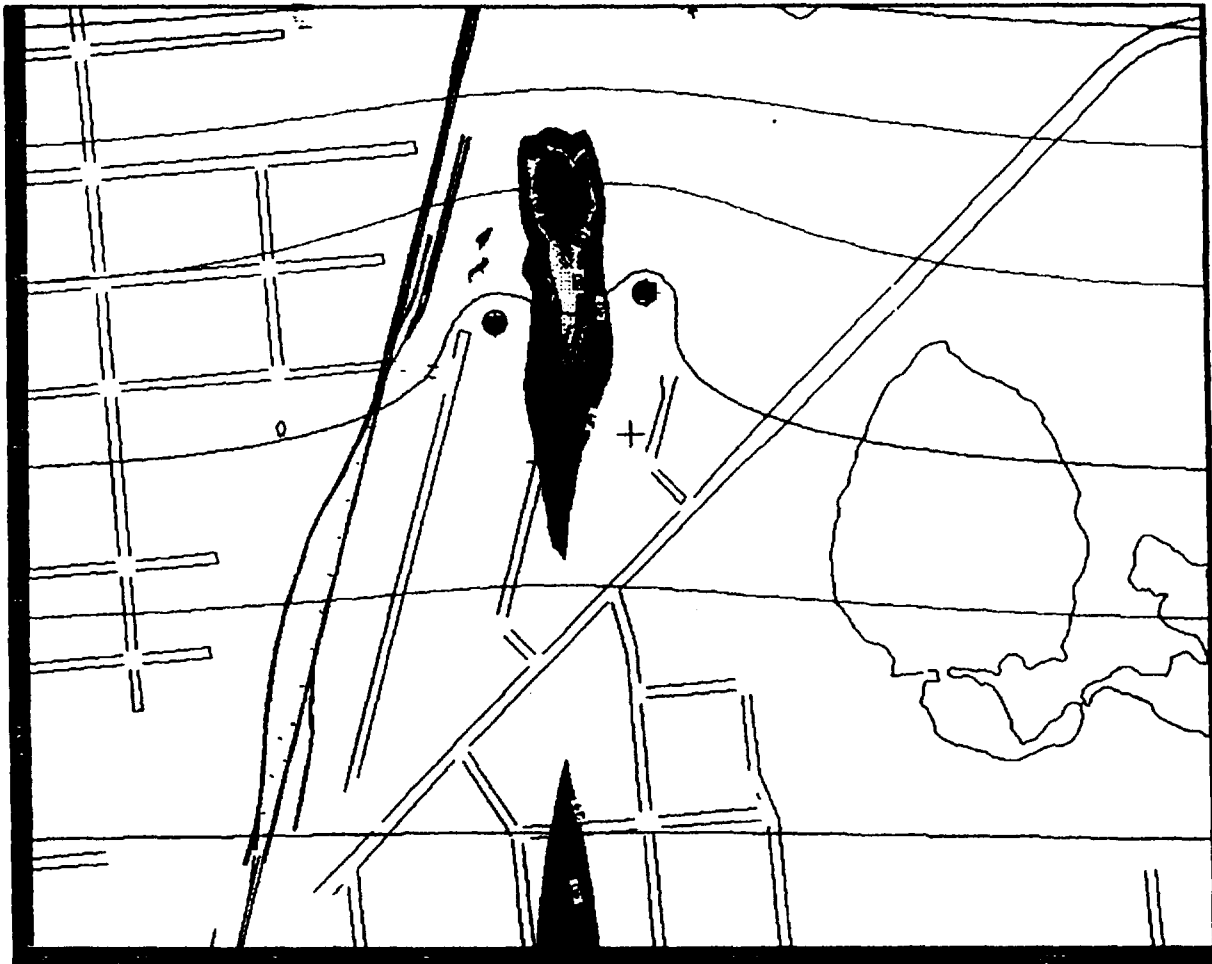
Figure 8: Predicted ammonia plume separation after 7 years of reduced summer pumping with a total Zone 1 pumping rate of 77 GPM (October to June)
