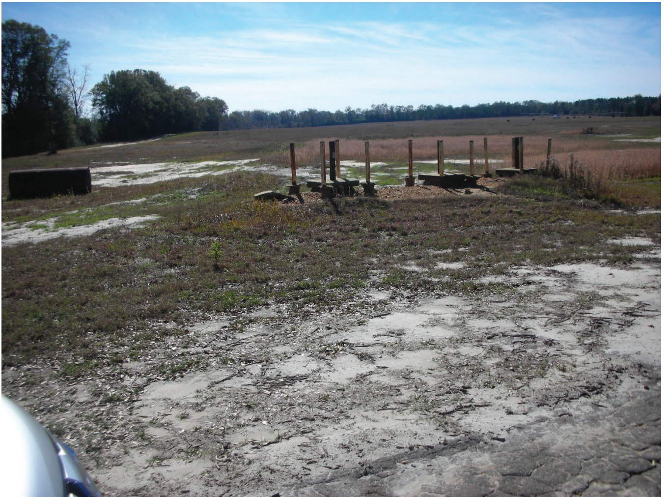
One cluster of monitoring wells on the site
