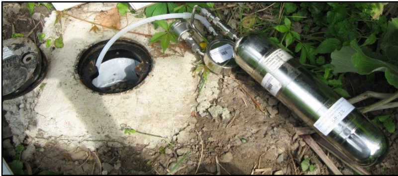
Soil gas sampling in progress
