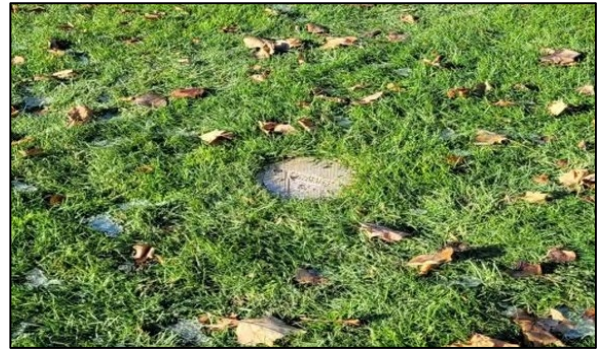
Completed soil gas sampling point
