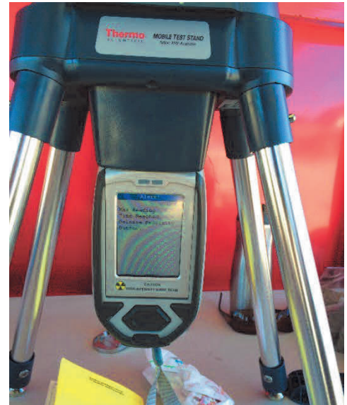
XRF stand with XRF attached.
