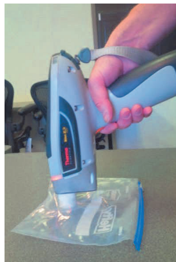
Figure 4: Reading standard with bag.
