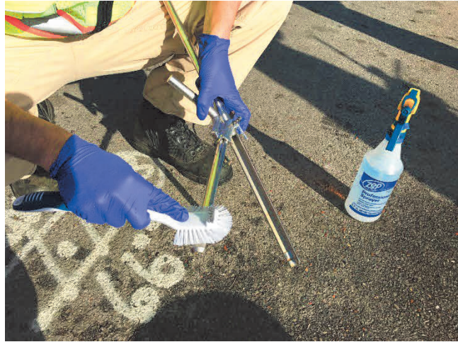
Decontamination of surface soil samplers.
