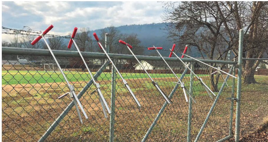
Surface soil samples drying after decontamination process.
