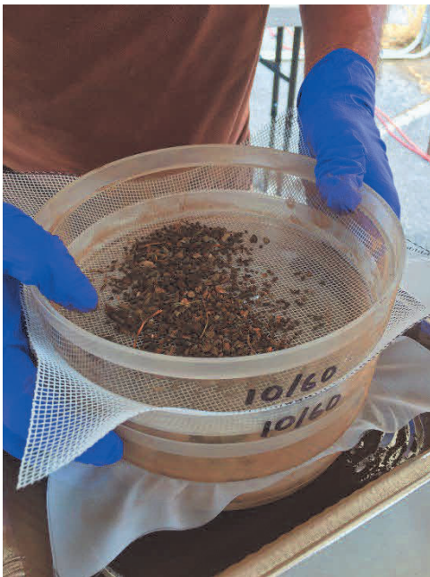
Stacked disposable sieves capturing the coarse fraction
