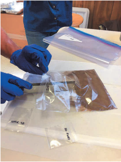
Subsamples taken from the parent fines soil sample.
