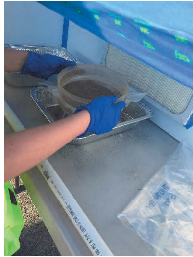
Soil samples being sieved under a fume hood.
