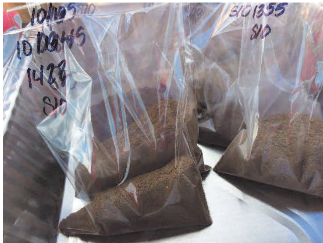
Sieved soil samples properly labeled and waiting XRF readings.
