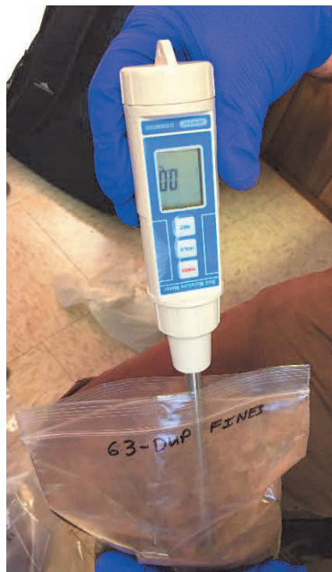
Figure 1: Obtaining a moisture reading using General Tools DSMM500 Precision Digital Soil Moisture Meter.
