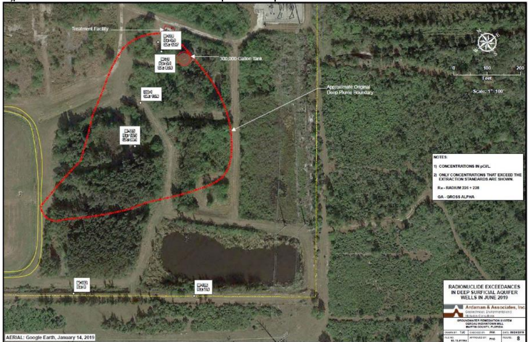
Figure I-5: June 2019 Radionuclide Exceedances in Deep Surficial Aquifer Wells
