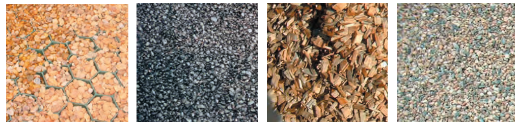
TRAIL SURFACE MATERIAL EXAMPLES: HONEYCOMB GRIDS, ASPHALT, MULCH, AND PEA GRAVEL
