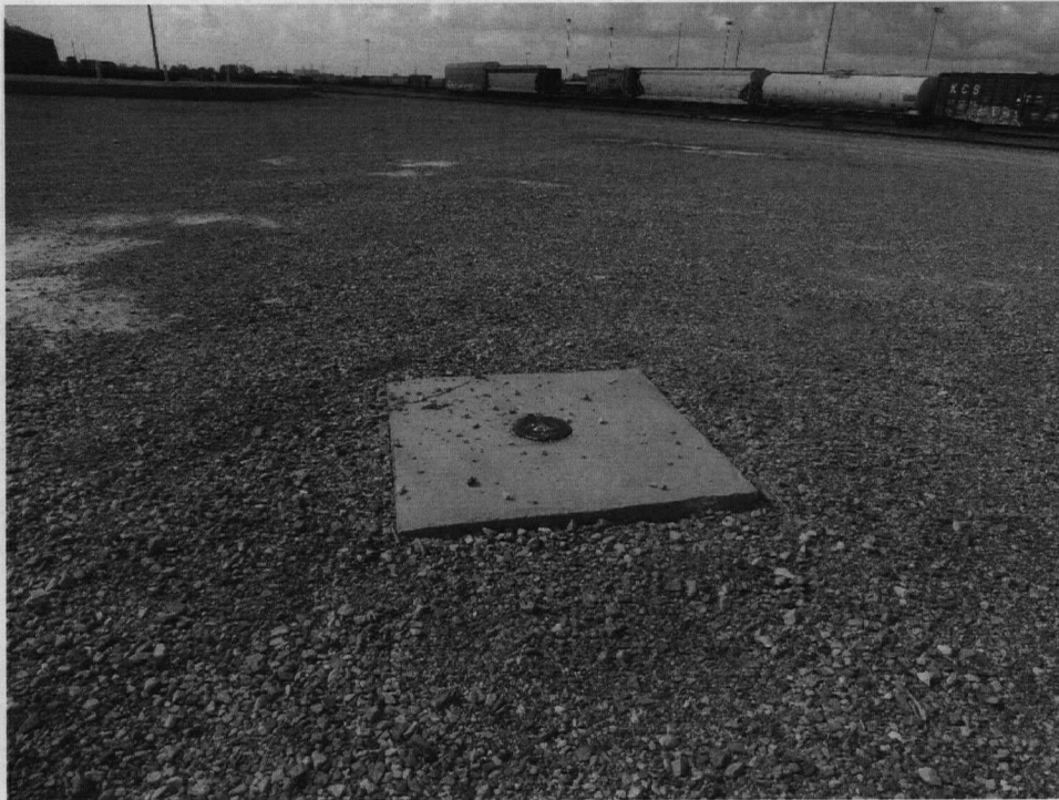
Flush mounted well with trains in background.
